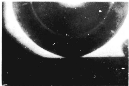
(c) Bubble diameter= 0.031 in. Contact angle: left= 14^\circ right= 18^\circ Voltage= 1.58 V
