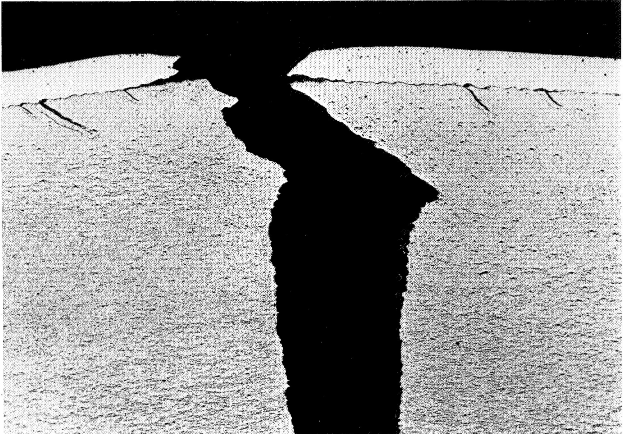
FIGURE 10. EXPLOSIVELY WELDED THICK-COMPOSITE BEND-TEST SAMPLE
