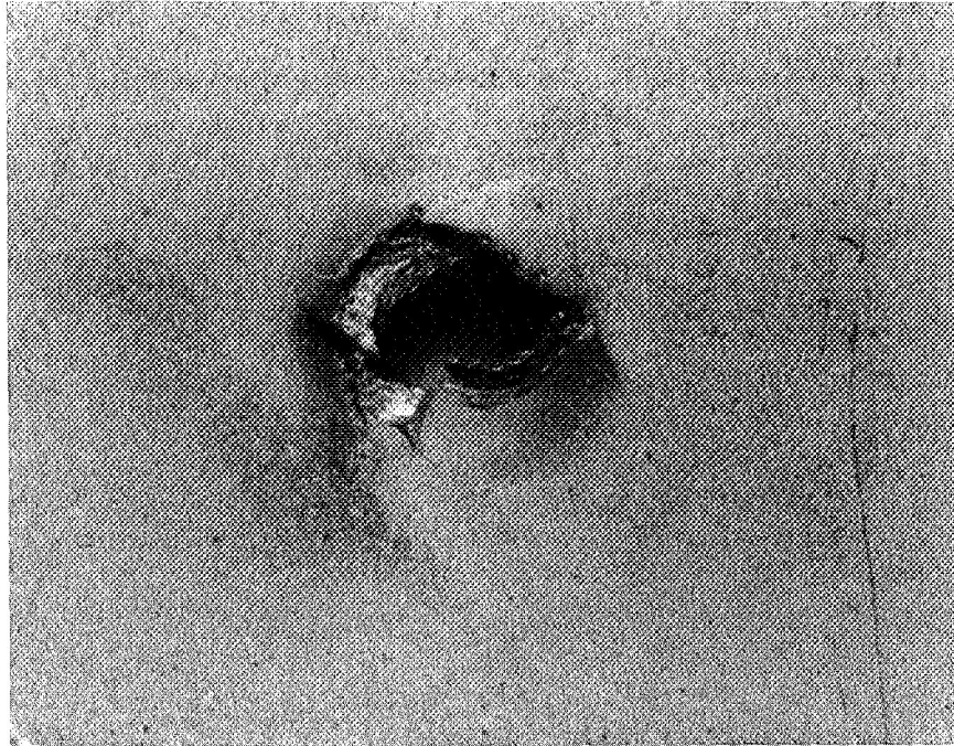
FIGURE 22. APPEARANCE OF SPECIMEN P-6 AFTER PUNCTURE-IMPACT EXPERIMENT
