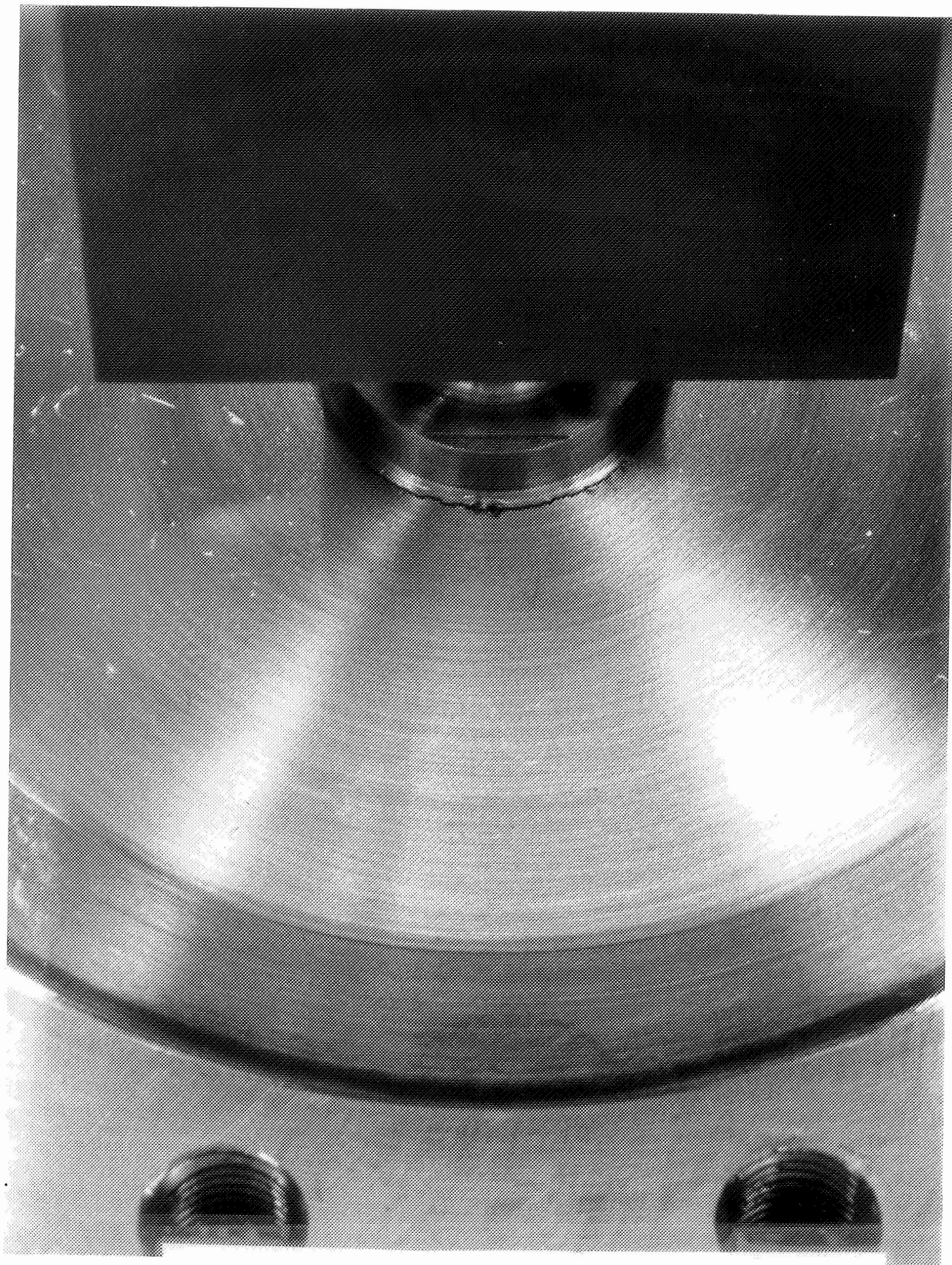
Diaphragm Failure Point As A Result of Destructive Burst Test
