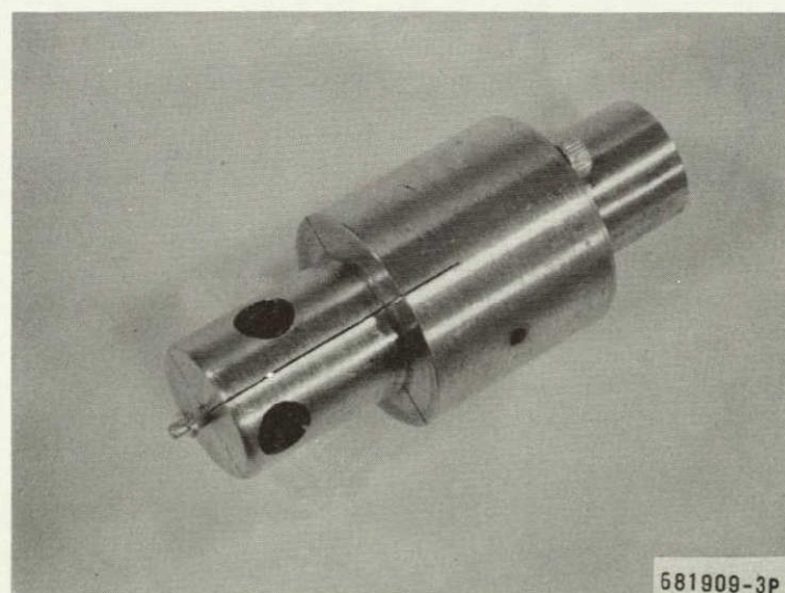
Figure 3-29. Test Fixture for Measuring Efficiency of GaAs "Flip-Chip" Schottky-barrier Diode
