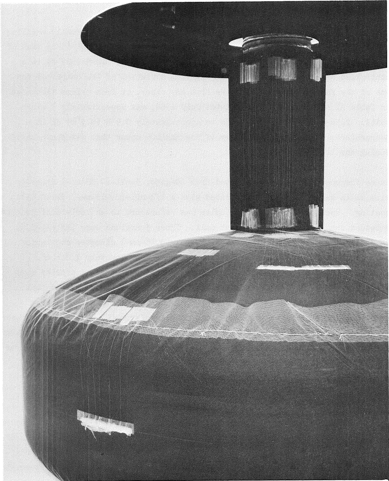
Fig. 3-8 Installation of Thermocouple Reference Wires
