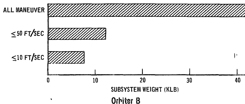
TURBOPUMP APS WEIGHT COMPARISON
