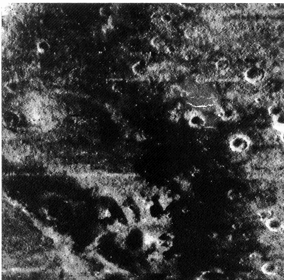
Figure 6. -The result of removing the streak noises from Figure 4. Note the presence of black and white spike noises scattered through the picture.
