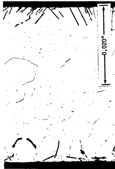
Welded in Helium & 250 ppm Air (F320842)
