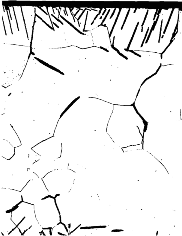
Exposed to NaK for 100 hrs at 1200°F (E951612)
