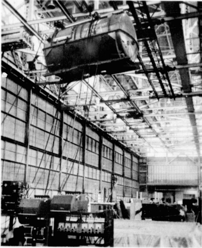
Fig. 23. Test Vehicle Shown Positioned for Impact in the Vertical Attitude Configuration--Pilot Compartment Airbag Restraint System
