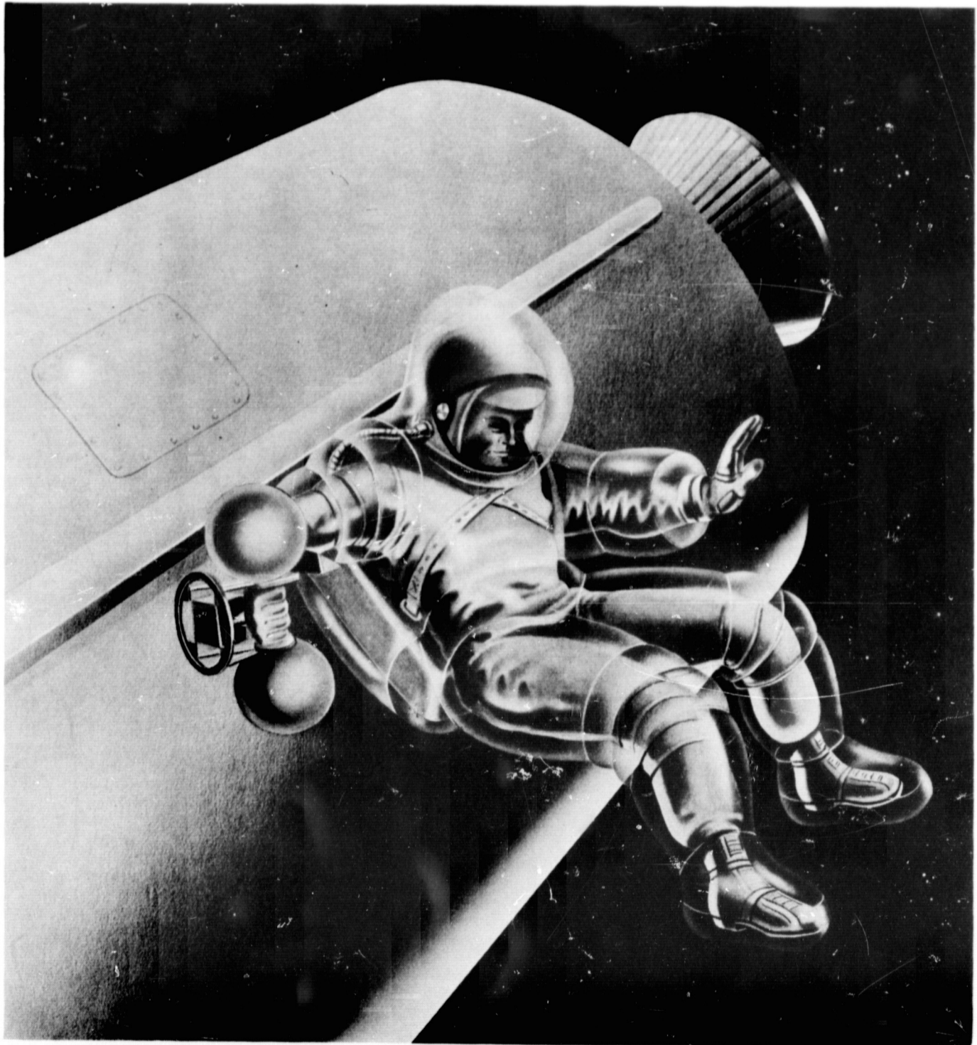
Fig. 68. Airbag Impact Protection System for the Extravehicular Maneuvering Astronaut
