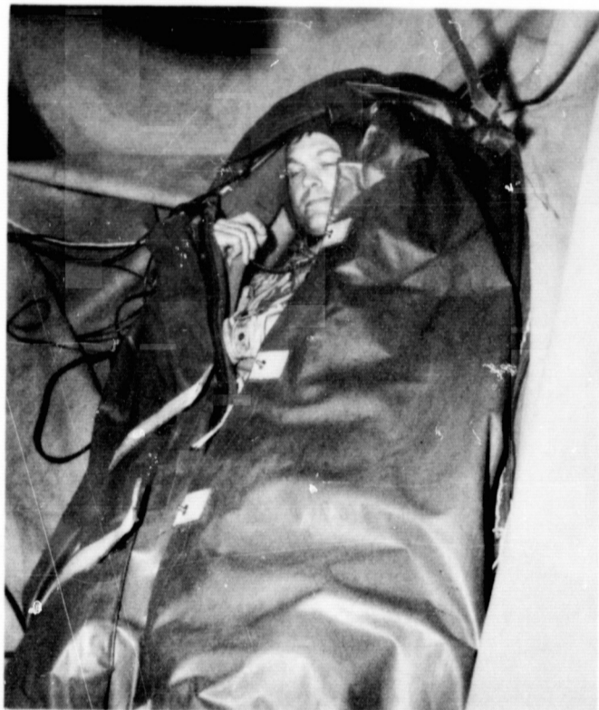
Fig. 18. Subject Positioned Inside "Bodybag" on Lower Airbag--45° Feet-Down and 45° Left-Side Configuration--Pilot Compartment Airbag Restraint System
