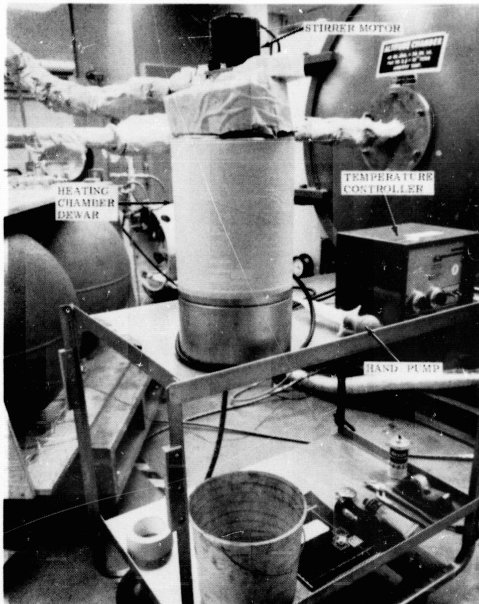
Figure 17. Inlet Fluid Temperature Control System
