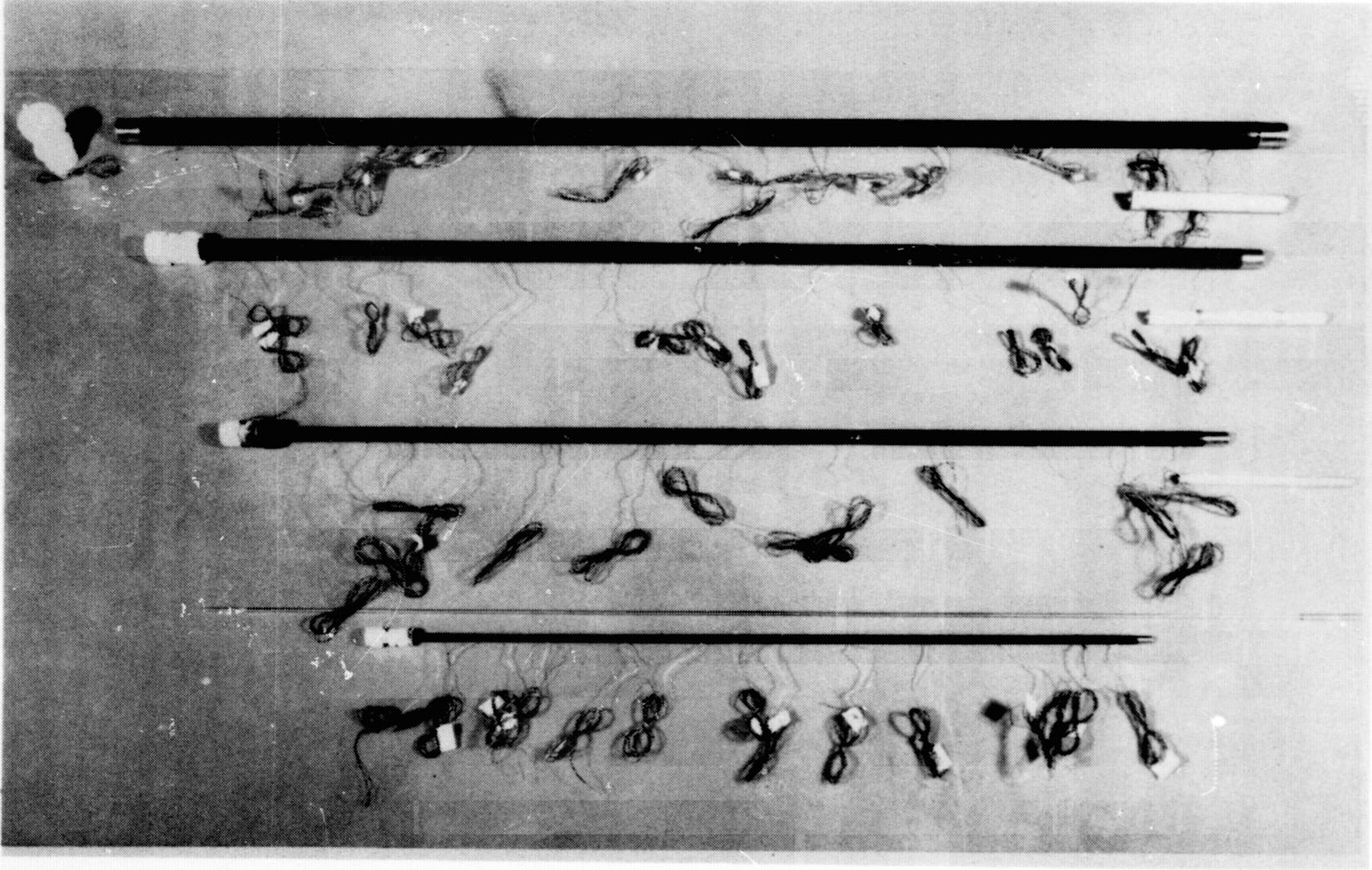
Figure 7. Stainless Steel Test Specimen Tubes and Plug Gages
