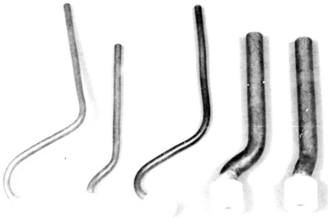
Figure 22. Copper Pipes with Sample "Ports" for Joint Integrity Testing
