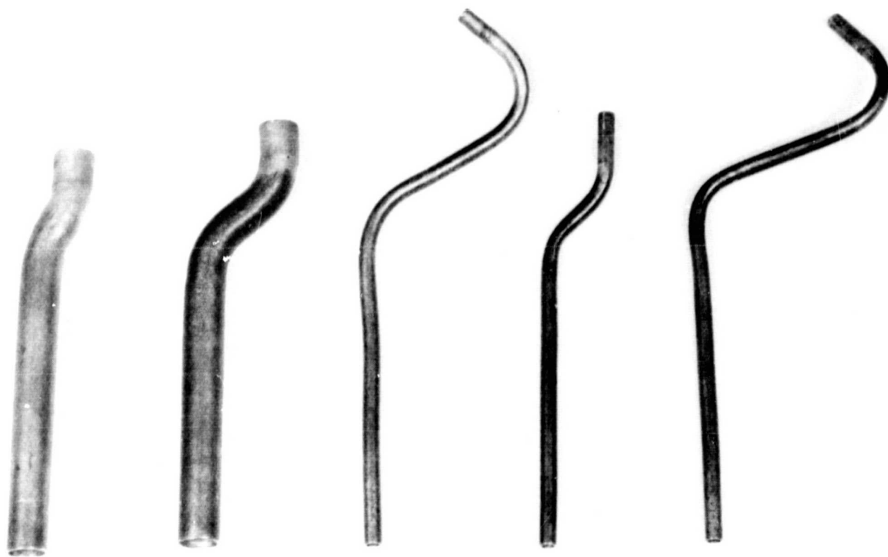
Figure 23. Copper Pipes After Removal of the Test Ports
