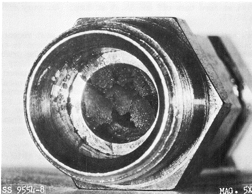
Solids Build Up In Urine Header Fitting
