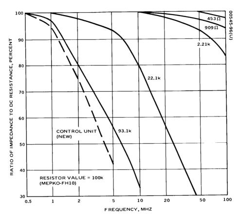
Figure 7-5. Impedance Versus Frequency of Five Carbon Film Resistors
