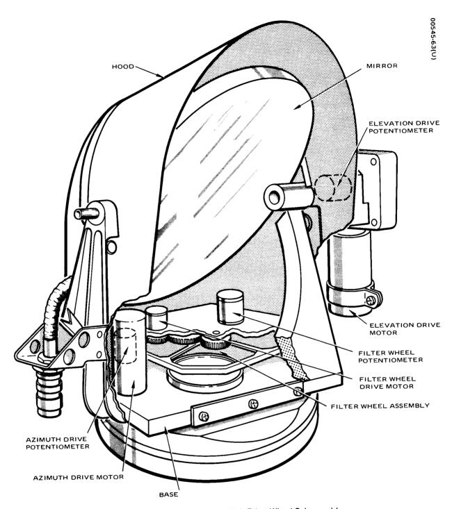
Figure 5-1. Mirror Assembly With Filter Wheel Subassembly
