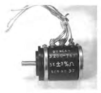
Figure 12-3. Surveyor III TV Potentiometer (Photo 00545-204)
