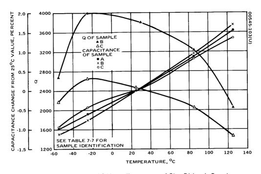
Figure 7-10. Capacitance and Q Versus Temperature of Glass Dielectric Capacitors
