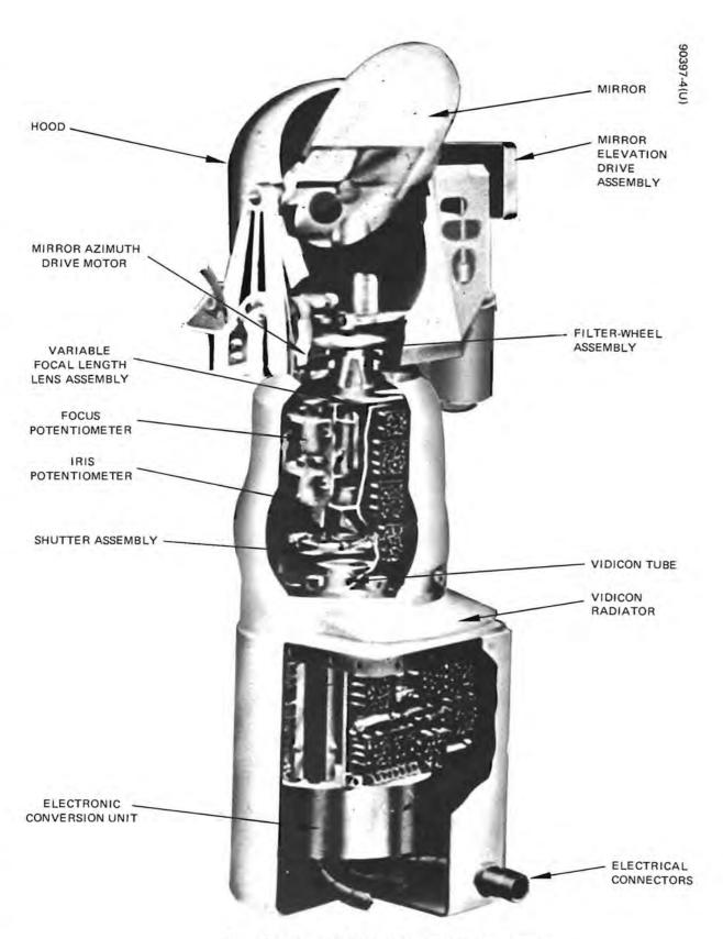
Figure 2-2. Cutaway View of Survey Television Camera
