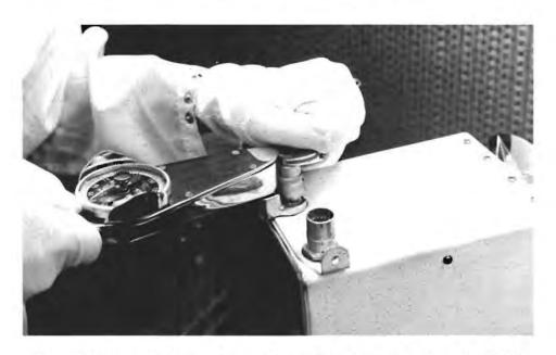
Figure 3-7. Removal of External Shroud Connector Retainer Nut (Photo 211-4000B)
