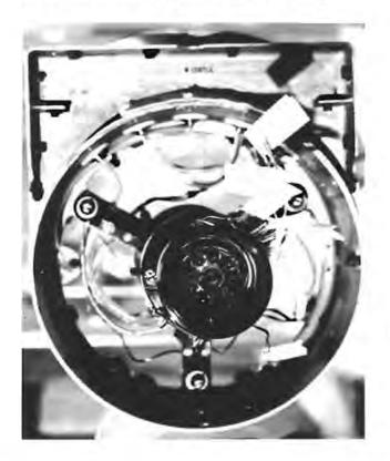
Figure 4-16. Rear View of Vidicon Housing Assembly (Photo 4R15892)
