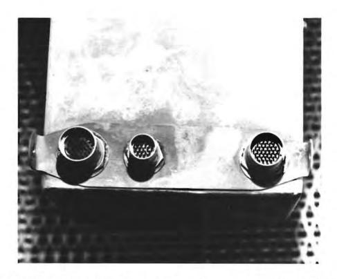
Figure 3-11. Lower Shroud After Removal of External Connectors (NASA Photo S-70-21142)
