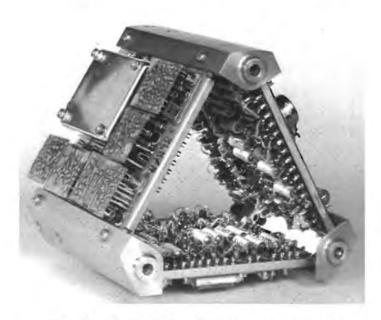
Figure 2-7. Electronic Circuits for Sweep, Control, and Amplification (Photo R98425)
