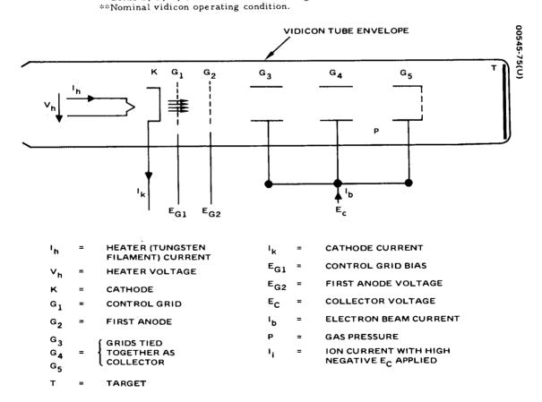
Figure 6-6. Diagrammatical Representation of Vidicon for Functional Tests
