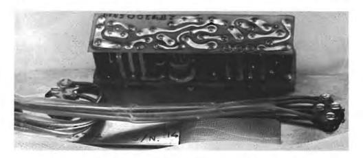
Figure 4-9. Star Mode Chassis A10 After Disassembly (Photo 4R15124)
