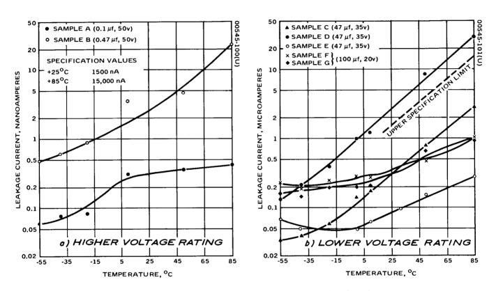
Figure 7-8. Leakage Current Versus Temperature of Tantalum Capacitors
