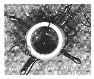
Figure 4-17, Vidicon Boron Nitride Collar (Photo 4R15891)
