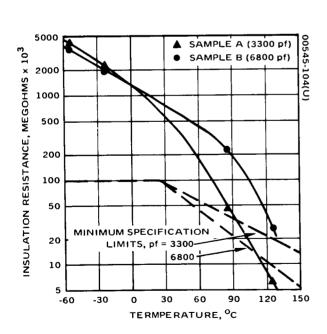
Figure 7-11. Insulation Resistance Versus Temperature of Dipped Mica Capacitors
