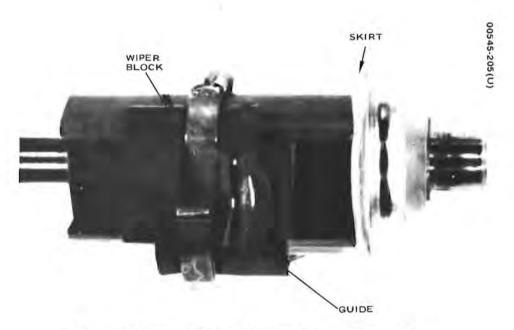
Figure 12-4. Wiper Block and Shaft Assembly of Potentiometer
