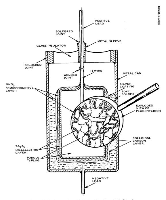
Figure 12-12. Construction of Solid Tantalum Electrolytic Capacitor
