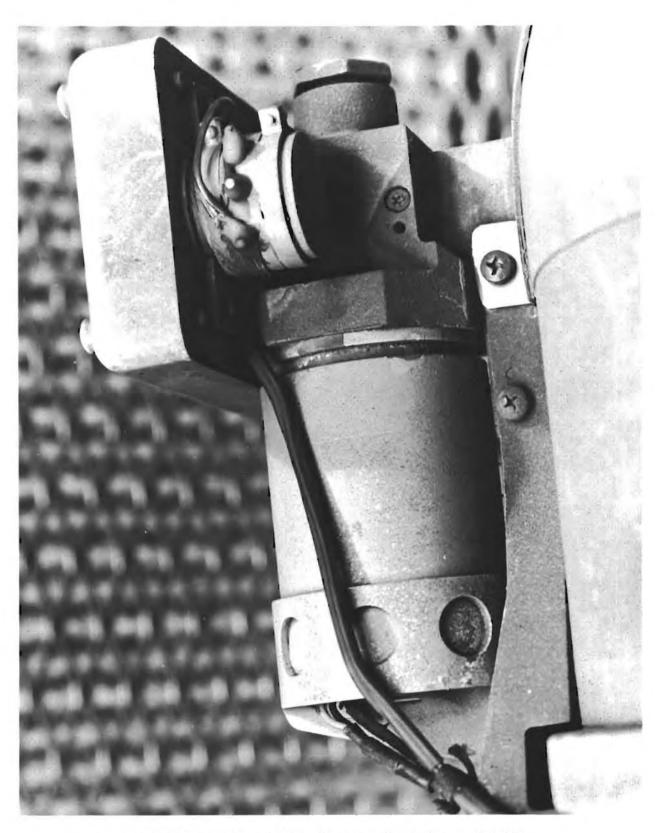
Figure 3-5. Mirror Elevation Drive Mechanism (NASA Photo S-70-21149)
