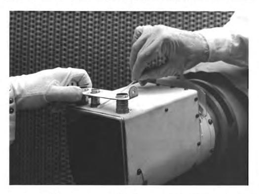
Figure 3-12. Removal of Connector Cable Support Bracket and Biological Assay (Photo 211-4001B)
