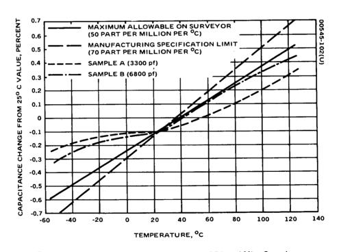
Figure 7-9. Capacitance Versus Temperature of Dipped Mica Capacitors
