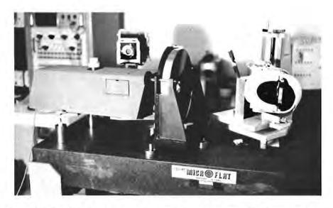
Figure 9-4. Test Setup for Original Measurement of Flatness of TV Mirror on Mirror Assembly (Photo 4R14065)
