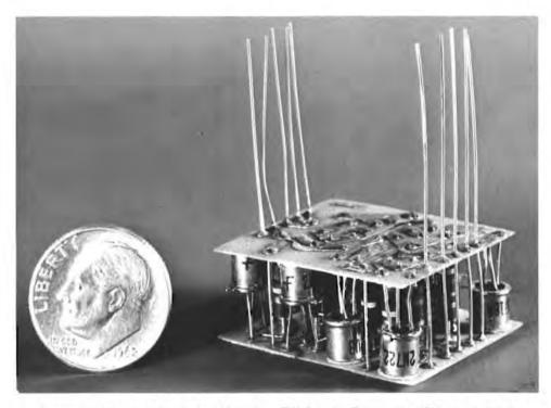
Figure 4-3. Typical Cordwood Module — TV Camera Electronics (Photo R87089)
