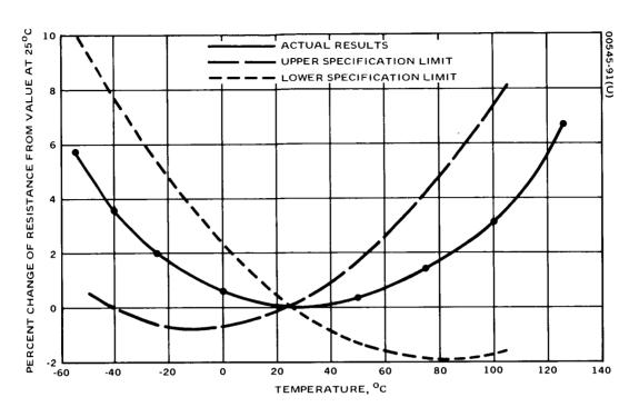
Figure 7-1. Resistance Versus Temperature of 1.5 Megohm Carbon Composition Resistor
