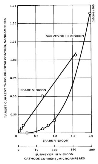
Figure 6-11. Measurement of Nesa Conductivity on Surveyor III and Spare Vidicon
