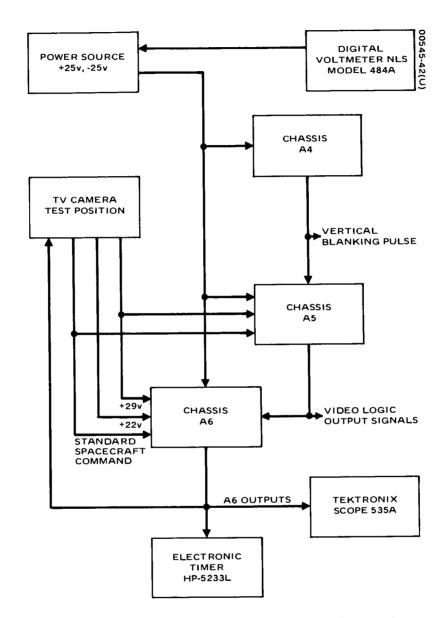
Figure 4-5. Test Setup for Functional Checkout of Chassis A6
