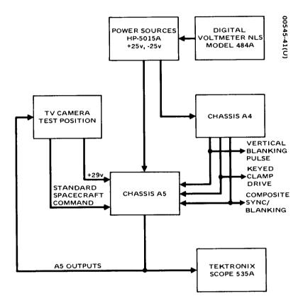
Figure 4-4. Test Setup for Functional Checkout of Chassis A 5
