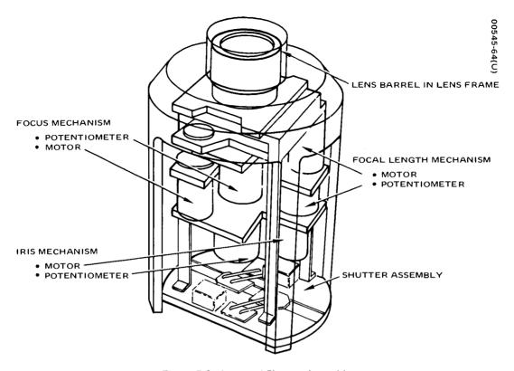
Figure 5-2. Lens and Shutter Assembly
