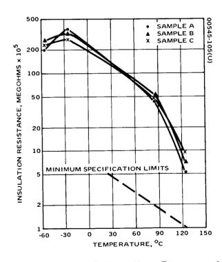
Figure 7-12. Insulation Resistance Versus Temperature of Glass Dielectric Capacitors
