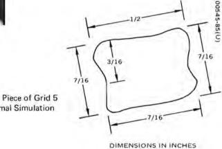
Figure 6-13. Torn Piece of Grid 5 Mesh During Thermal Simulation Test
