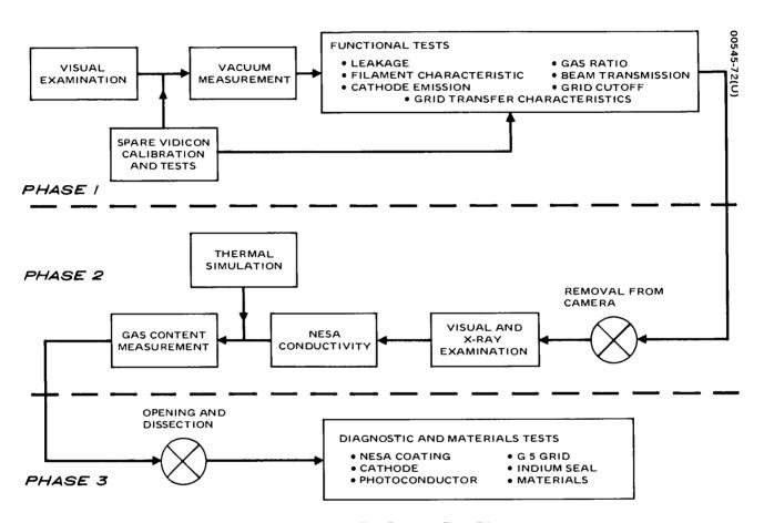
Figure 6-4. Vidicon Test Program Flow Diagram
