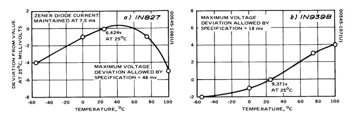
Figure 7-13. Voltage Versus Temperature of Zener Diodes
