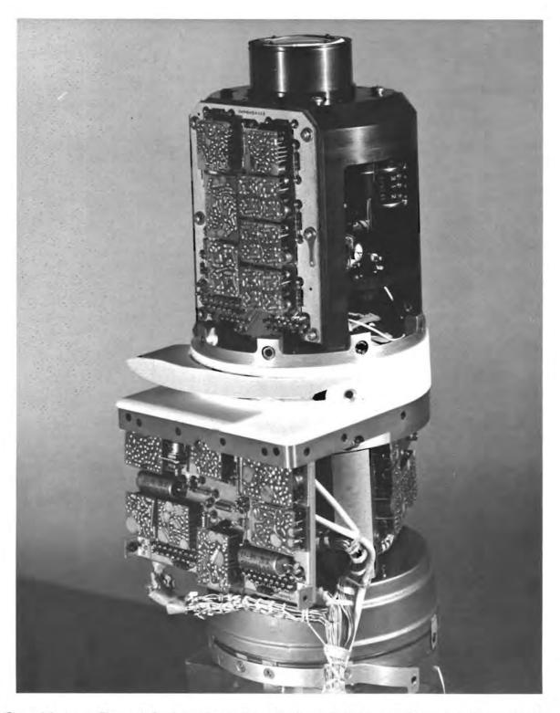
Figure 2-3. Lower Electronic Portion of Survey Television Camera With Mirror Unit Removed (Photo R96128)
