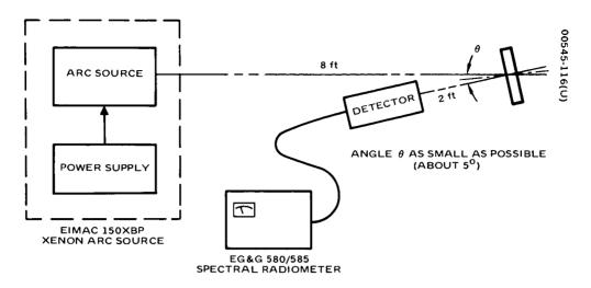
Figure 9-1. Experiment Setup for Specular Reflectance Measurements of TV Mirror
