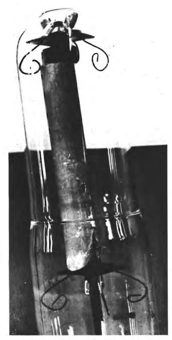
Figure 11-2. White Painted Tube Section Returned From Moon in SESC in Quartz Vacuum Chamber (Photo 00545-292)
