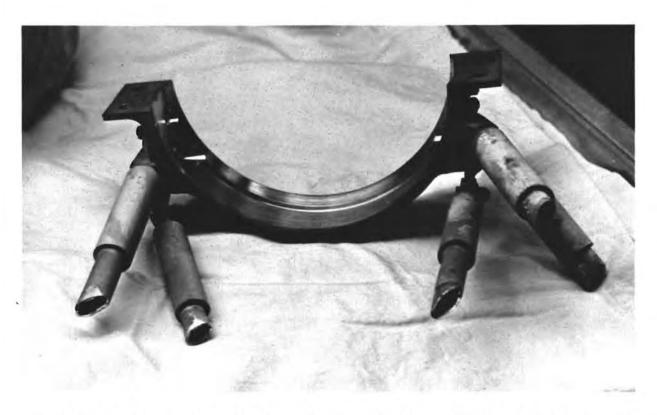
Figure 3-8. Camera Mounting Collar – Left Section With Remnants of Support Struts (NASA Photo S-70-21157)
