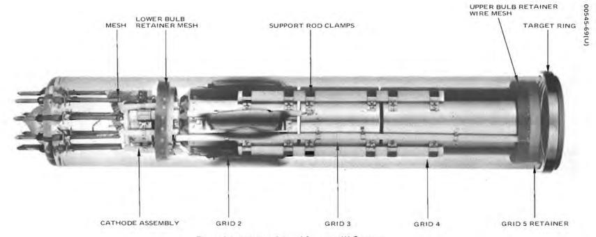
Figure 6-1. Vidicon Tube of Surveyor III Camera
