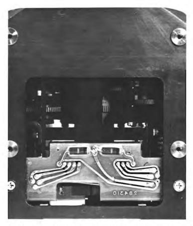
Figure 4-8. Front View of Lens Support Structure and Shutter Assembly (Photo 4R14816)
