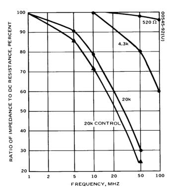
Figure 7-2. Impedance Versus Frequency of Three Carbon Composition Resistors
