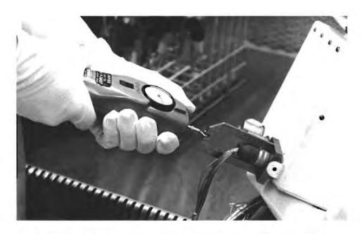
Figure 3-6. Removal of External Lower Shroud Connector (Photo 211-3999B)
