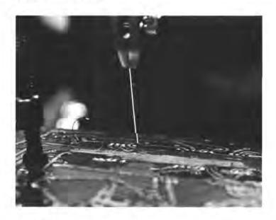
Figure 10-6. Conductor Peel Strength Test Setup (Photo 00545-177)
