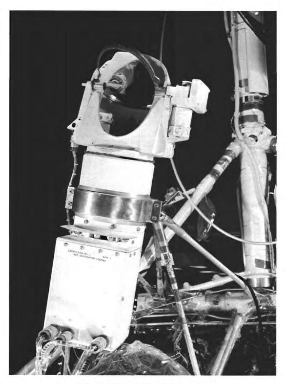
Figure 2-1. Survey Television Camera (Photo A07257)
