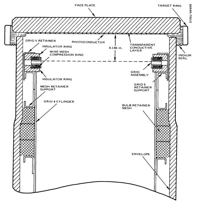
Figure 6-2. Cross-Sectional View of Front Portion of Vidicon
