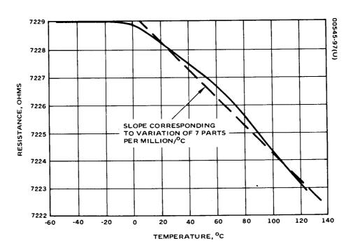
Figure 7-6. Resistance Versus Temperature of Precision Wire-Wound Resistor
