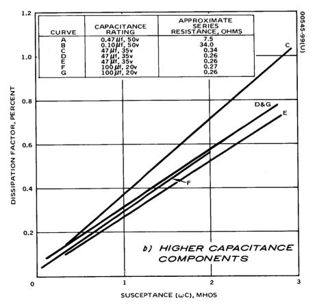
Figure 7-7. Dissipation Factor Versus Susceptance of Solid Tantalum Capacitors
