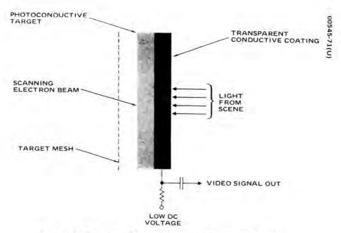
Figure 6-3. Functional Diagram of Vidicon Transducing Process
