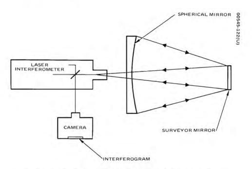
Figure 9-5. Illustration of Double-Pass Interference of Flatness Measurement
