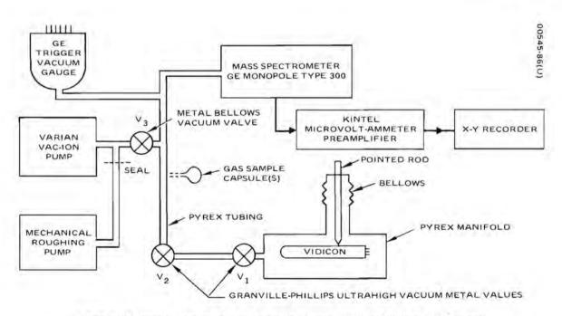
Figure 6-14. Block Diagram of Test Setup for Measurement of Vidicon Gas Content
