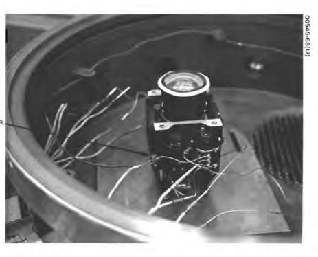
THERMOCOUPLE CONNECTED TO LENS FRAME, UNDER WASHER . AND SCREW HEAD
