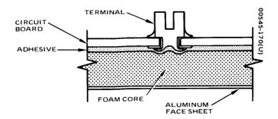
Figure 10-1. Etched Circut Board Sandwich Construction
