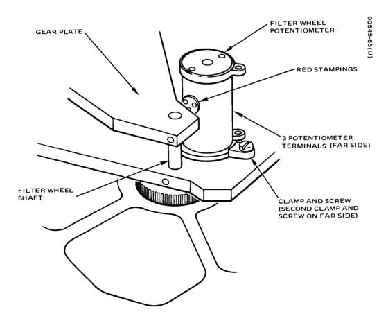
Figure 5-3, Removal of Filter Wheel Potentiometer
