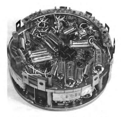
Figure 2-6. Electronic Conversion Unit (Photo R98455)
