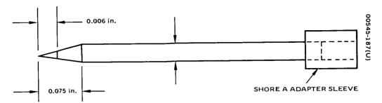
Figure 10-13. Modified Probe for Shore A Tester for Hardness of Adhesives
