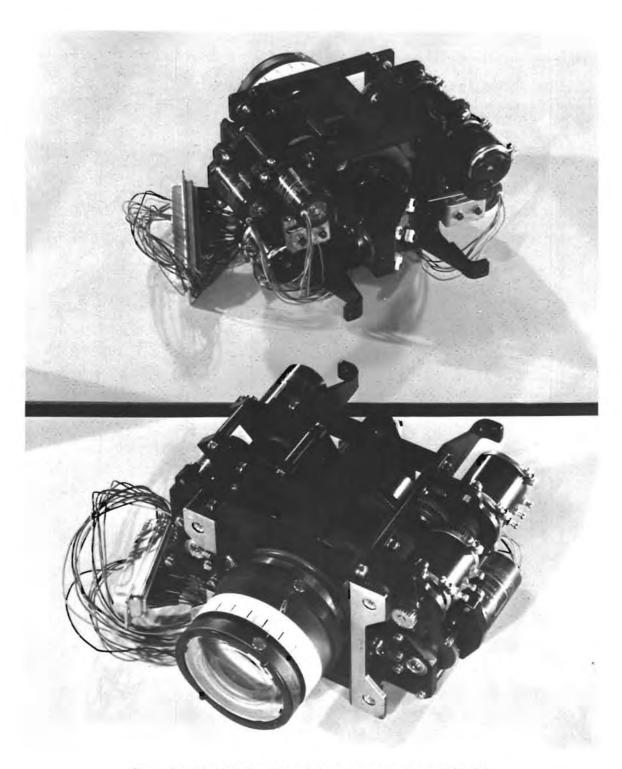
Figure 2-4. Variable Focal Length Lens Assembly (Photo R97597)
