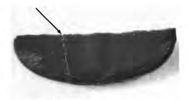
Figure 12-5. Cracked and Broken Off Guide Block of Filter Wheel Potentiometer (30X Magnification) (Photo 00545-206)
