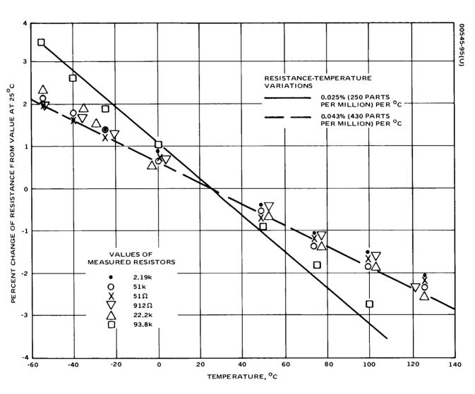
Figure 7-4. Resistance Versus Temperature of Six Carbon Film Resistors
