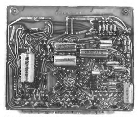
Figure 4-14. Etched Braided Circuit Board Side of Chassis A6 (Photo 4R15698)
