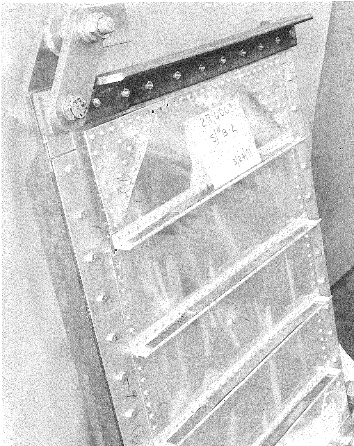
FIGURE 7-8. DETAIL OF SHEAR FAILURE OF BORON/EPOXY REINFORCED STRINGER TEST PANEL.
