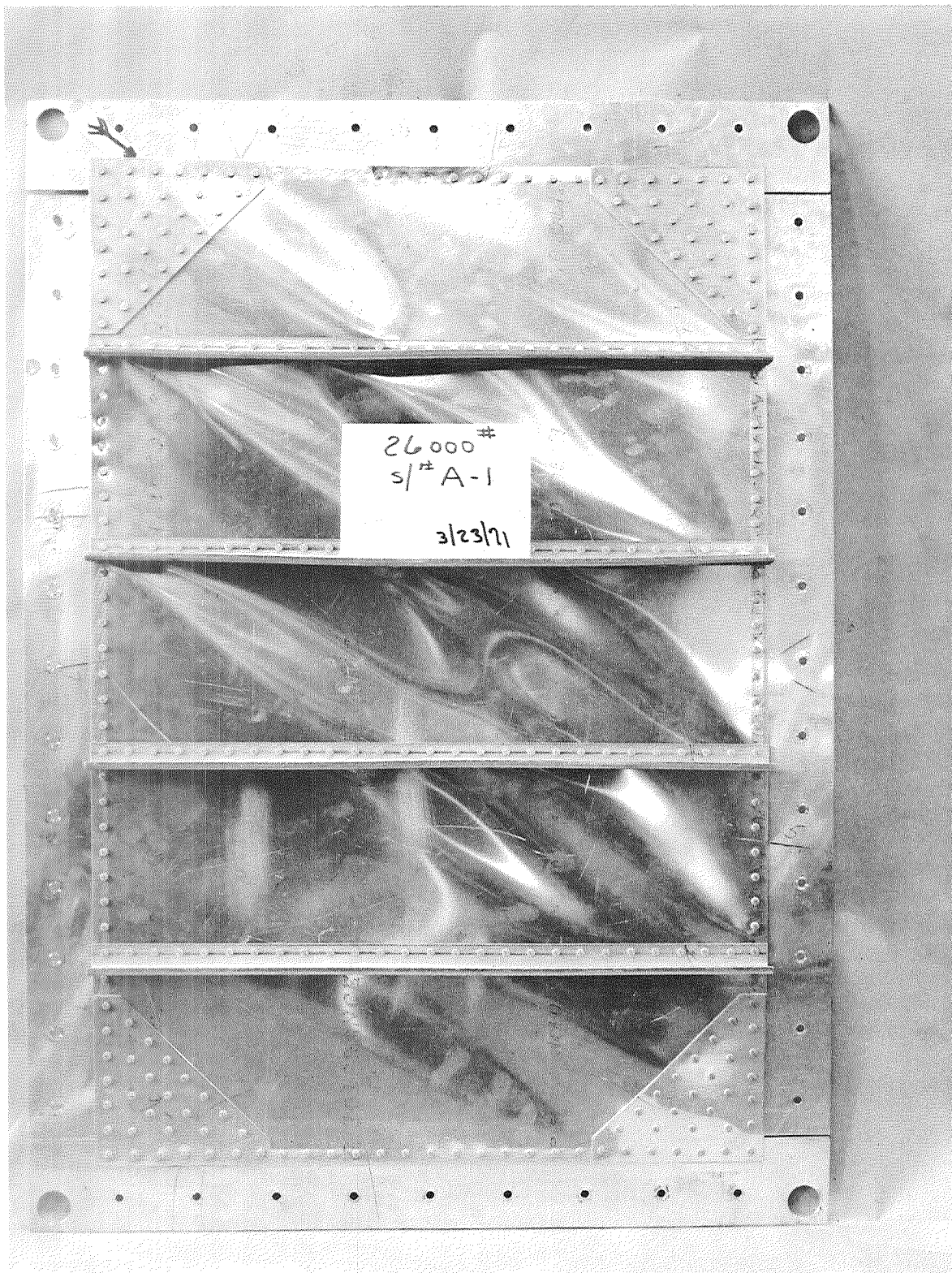
FIGURE 7-6. SHEAR FAILURE OF NONREINFORCED TEST PANEL.
