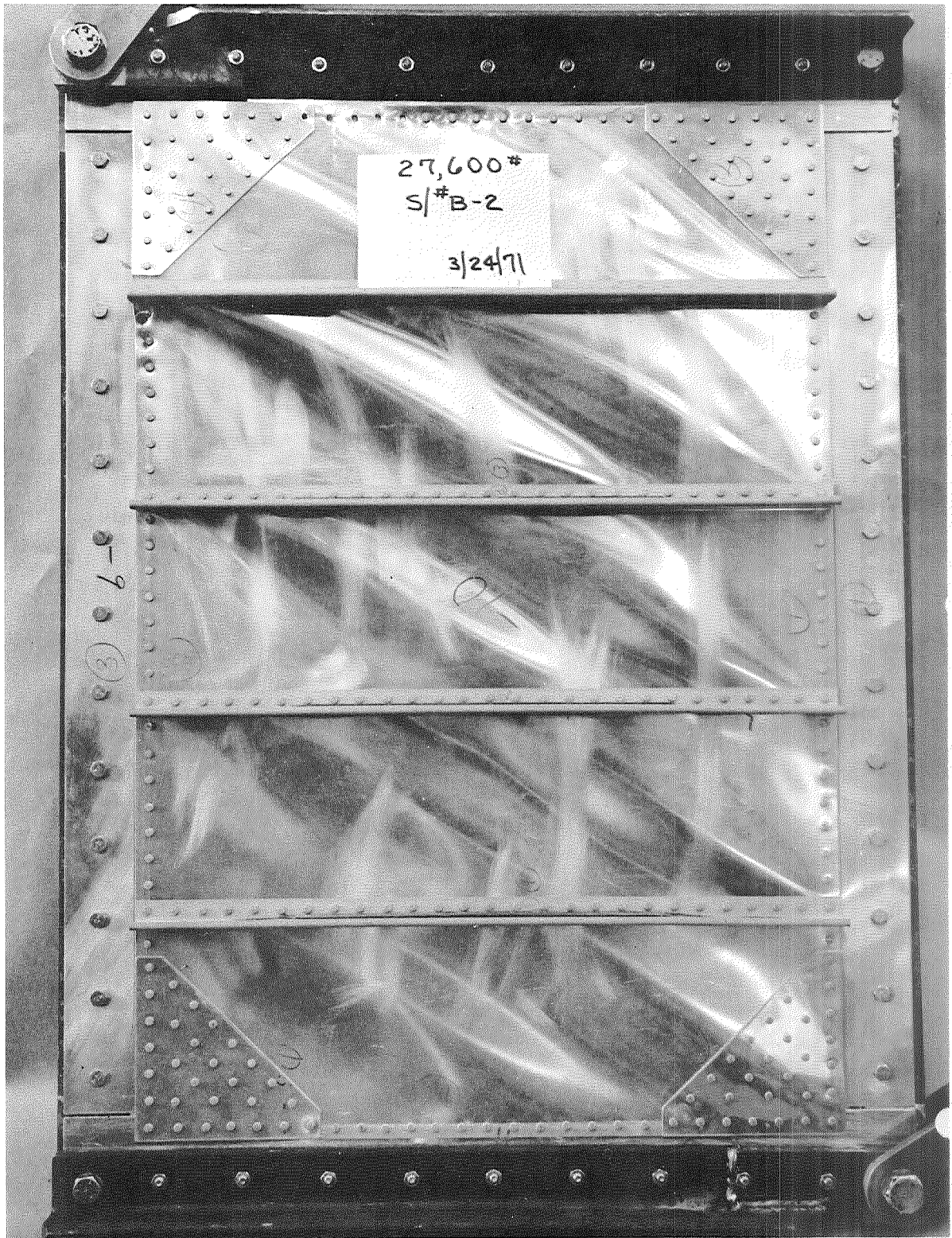
FIGURE 7-7. SHEAR FAILURE OF BORON/EPOXY REINFORCED STRINGER TEST PANEL.
