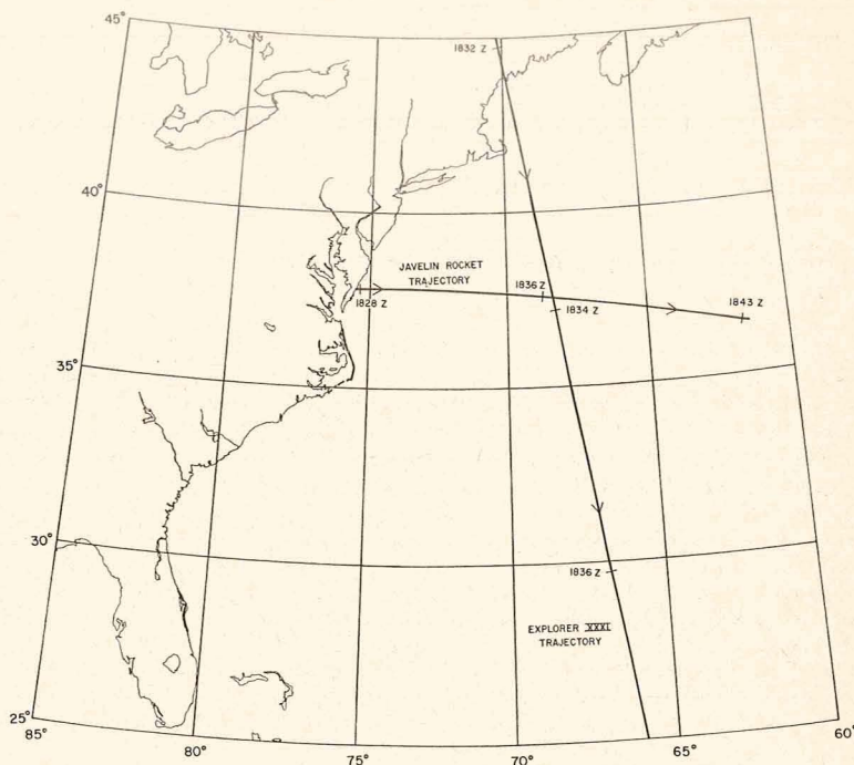
Fig. 1. Trajectories of Javelin rocket and Explorer 31 satellite showing direction of travel and local times. Satellite altitude at crossing of trajectories was 972 km; rocket was at peak altitude, 723 km.
