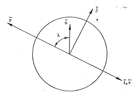
FIGURE 5.2. VECTOR GEOMETRY FOR REFERENCE RECTILINEAR ORBIT RELATIVE TO OBLATE CENTRAL BODY.
