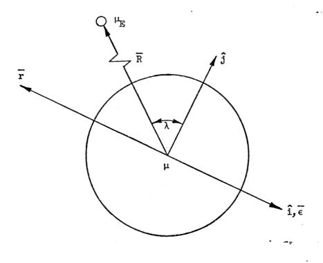
FIGURE 5.3. VECTOR GEOMETRY FOR REFERENCE RECTILINEAR ORBITS RELATIVE TO FIXED EXTERNAL BODY.
