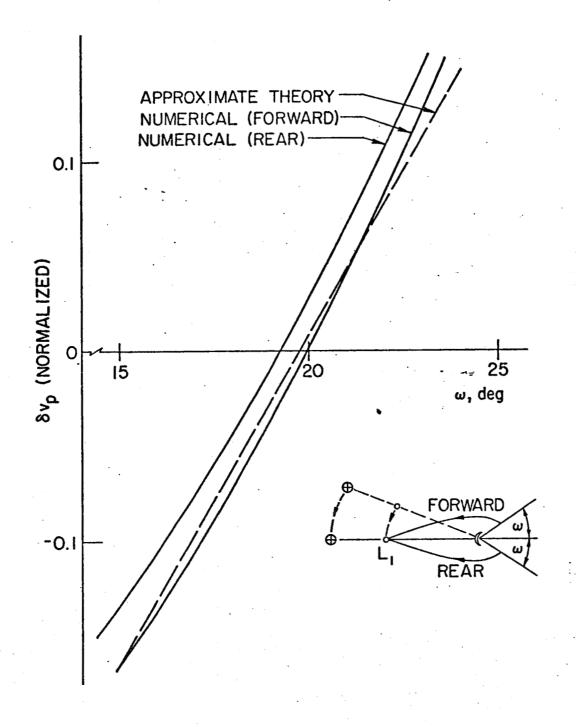
FIGURE 6.2. VARIATION PARABOLIC VELOCITY AT PERILUNE VS ORIENTATION ANGLE  $\,\omega\,$  .
