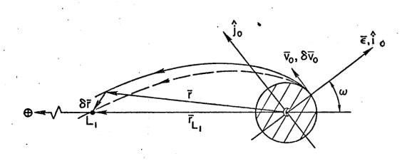
FIGURE 6.1 VECTOR GEOMETRY FOR REFERENCE PARABOLA RELATIVE TO EARTHMOON LINE
