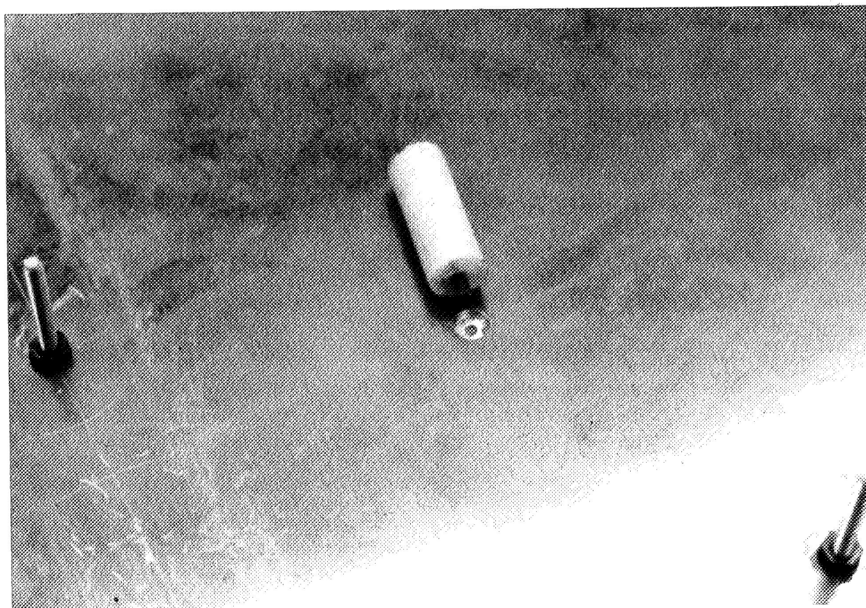
Figure 22.- Screw Head Recessed in Tooling
