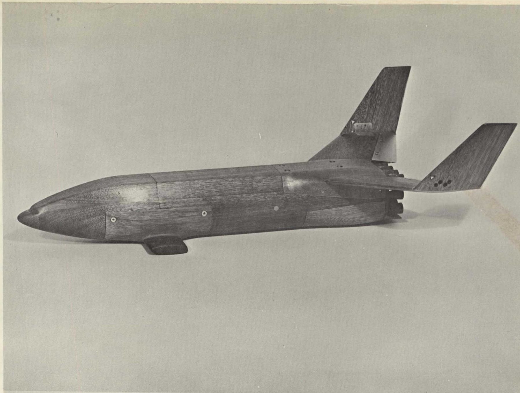
FIGURE 10. (a) B_1N_1W_1E_1V_1J_1 (SIDE VIEW) MDC(WD) SPACE SHUTTLE 1% BOOSTER SCALE MODEL JET FLAP CANARD HIGH WING CONFIGURATION
