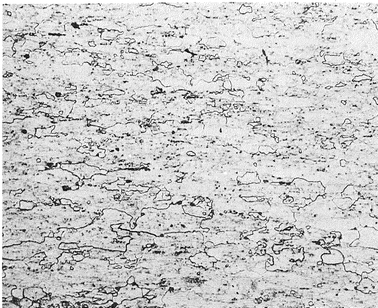
(a) Sheet surface, rolling direction is horizontal
