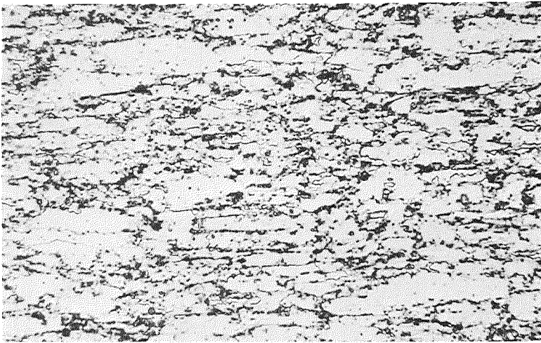
(a) Sheet surface, rolling direction is horizontal
