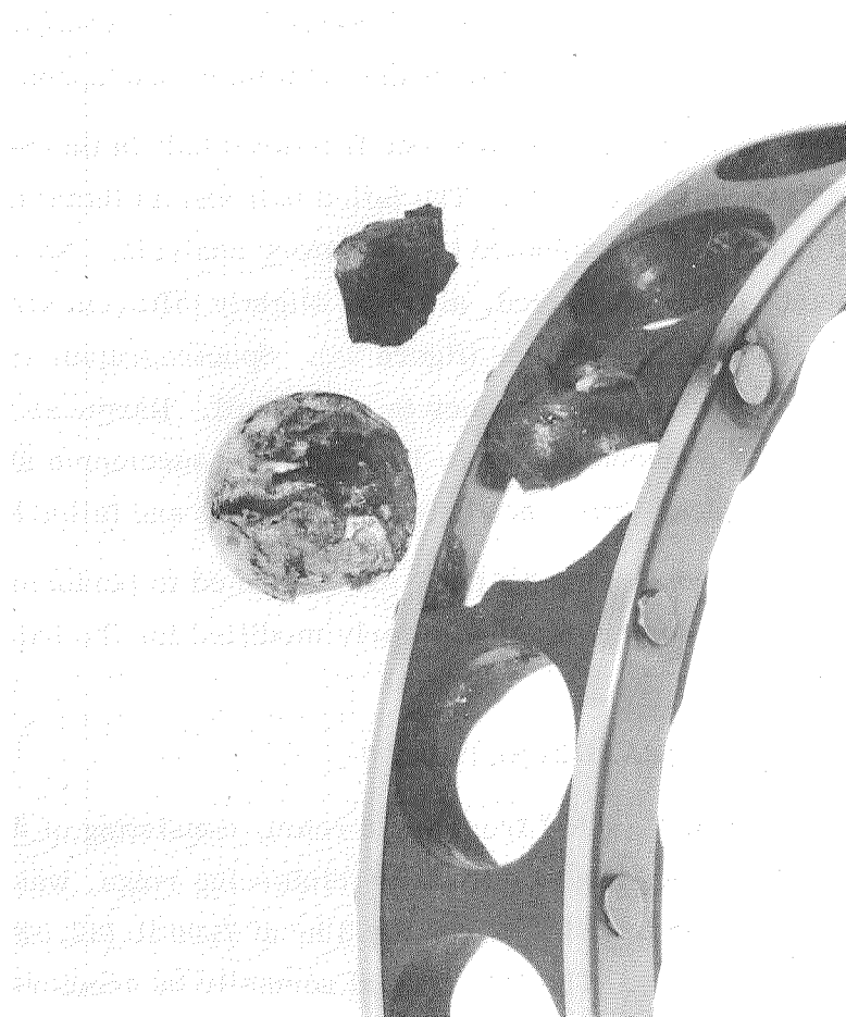
Figure 33. Test No. 14 Cage DKJ 6202, Bearings 2137774, S/N L10, With Fractured Star J Ball and Damage to Cage
