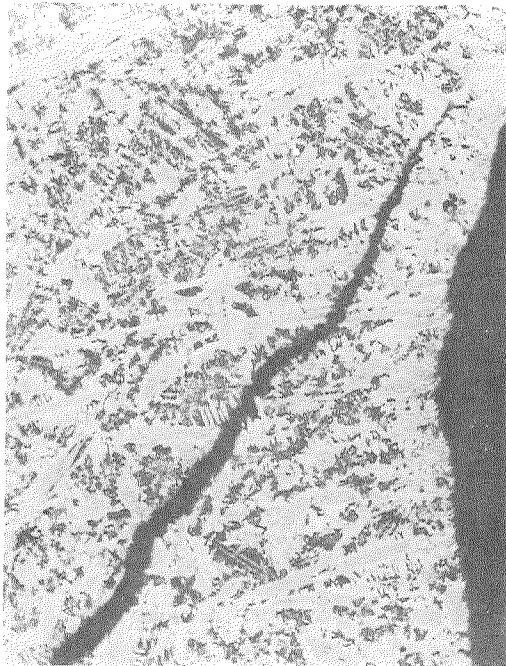
Microstructure of the Failed Ball at the Ball Outer Edge
