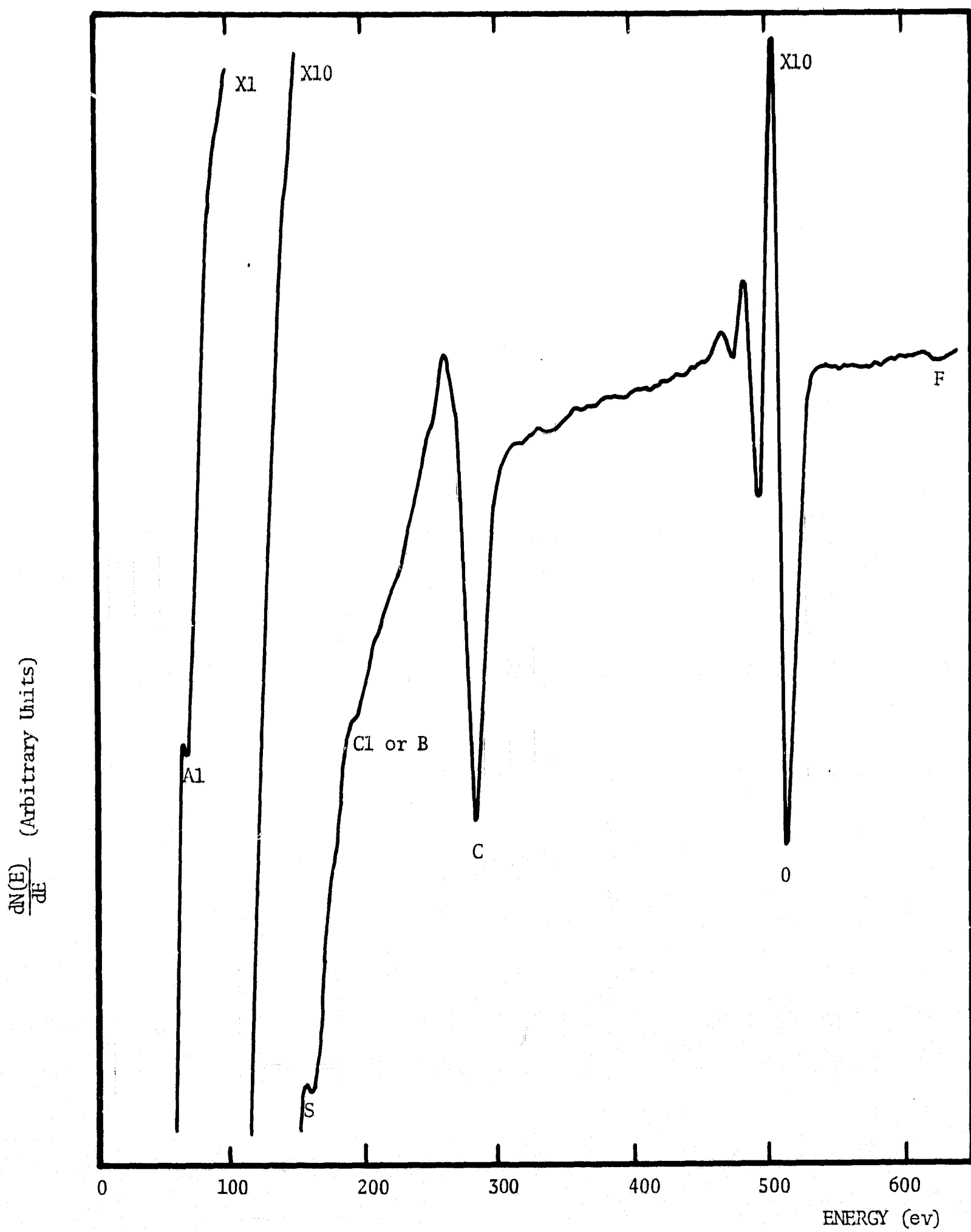
FIGURE 25. TYPICAL WAFER AFTER Al MASK, PHOTORESIST REMOVED
