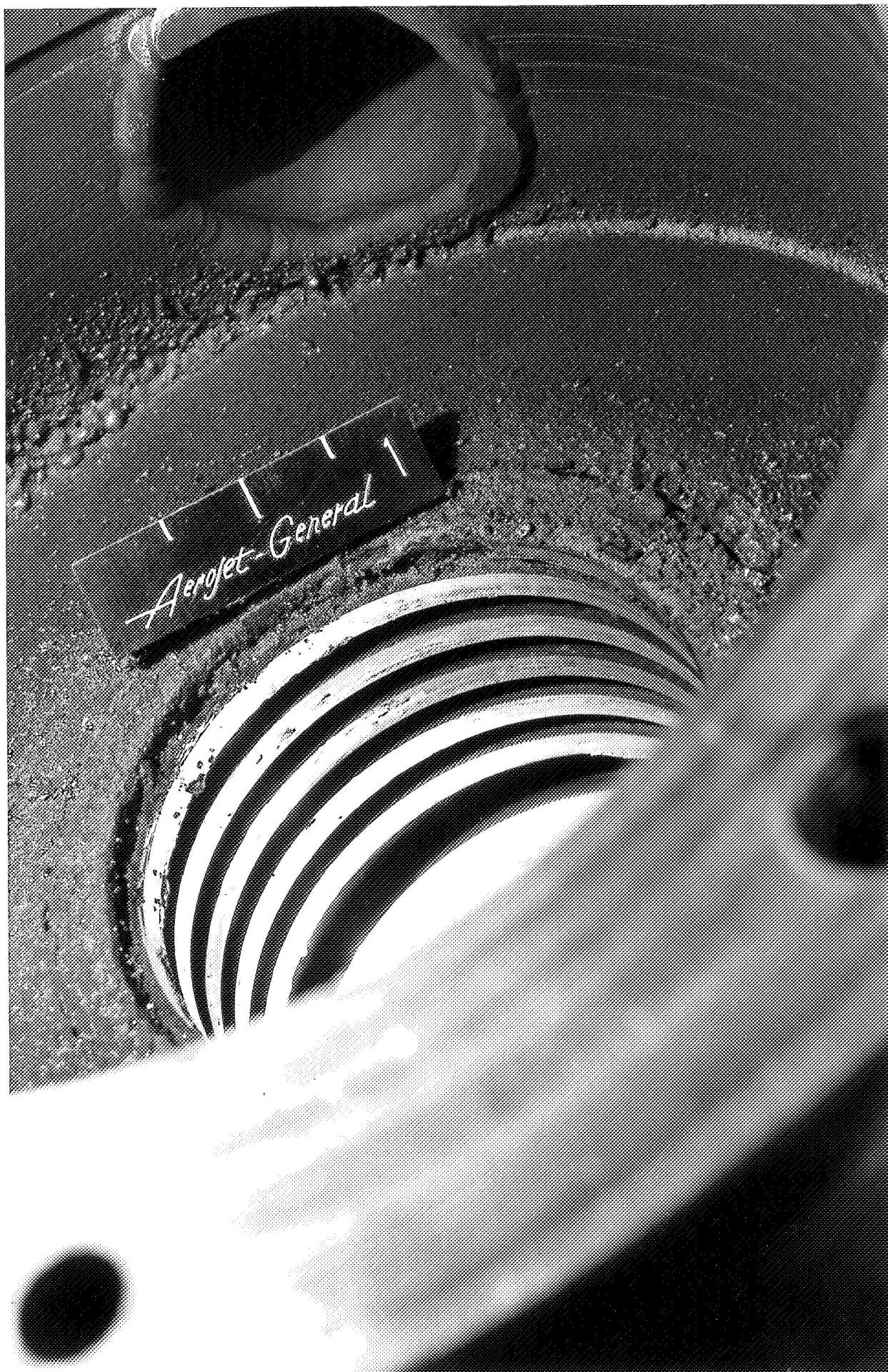
MOD-C TESTER (REFERENCE UNIT) HOUSING, MOLECULAR PUMP GROOVES 1683.9 HRS OPERATION 3/13/69
