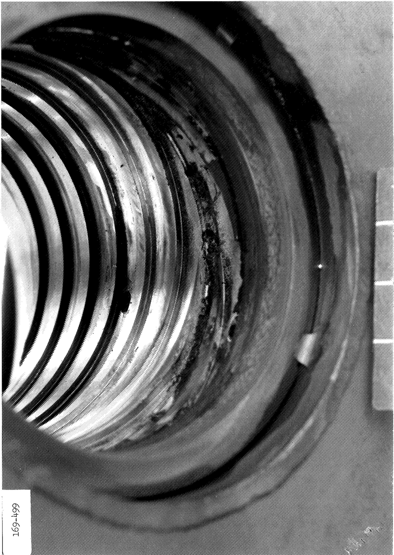
MOD-C (MAJOR MOD) VISCO PUMP HOUSING (ii) AFTER 421 HRS. 1-16-69
