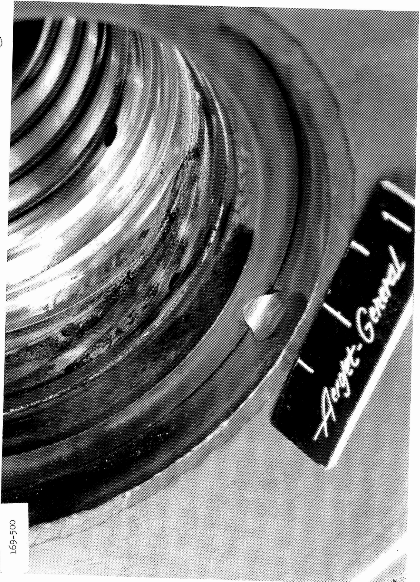
MOD-C (MAJOR MOD) VISCO PUMP HOUSING (i) AFTER 421 HRS. 1-16-69
