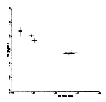
FIGURE 12 Plot of log (B<sub>S</sub> cos e) versus log (cos i cos e) for  $\lambda$  = 1.47 µm and  $\alpha$  = 5.2. The data plotted are for points observed along the STB.
