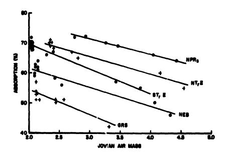
FIGURE 4 Percent absorption of NH $_3$  as a function of Jovian air mass for points observed along individual belts, zones, or following a spot across the disk. The percent absorption was computed using the data obtained from the 1.47, 1.50 and 1.53  $\mu$ m passband cell (see Table 1).
