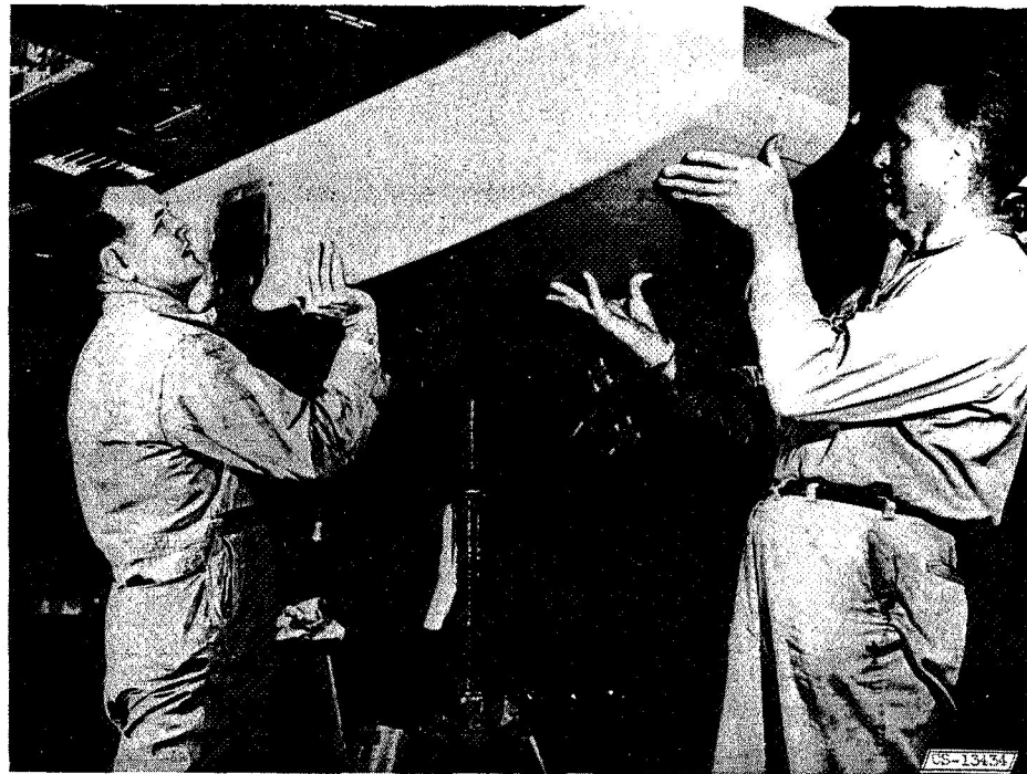
Figure 9. - Heat-exchanger air scoop.
