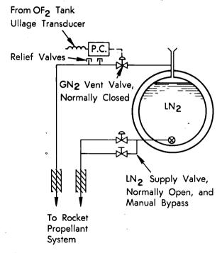
in the  $OF_2$  tank as the liquid temperature and vapor pressure of the  $OF_2$  rises or falls. The vent valve cycles slowly between an open and closed position to maintain  $OF_2$  temperature somewhat above or below the setpoint.
