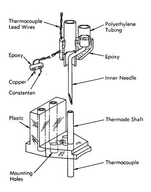
possible; a small amount of wetting agent added to the water bath also tends to reduce resistance to flow. Once suitable flow rates are obtained, the thermode is calibrated by monitoring tip temperature over a range of water bath temperatures.
