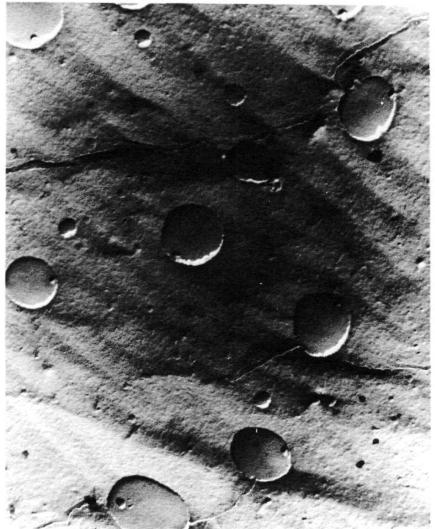
Fig. 2. Surface replica of an undoped solar cell irradiated with 10^{11} neutrons/cm 2
