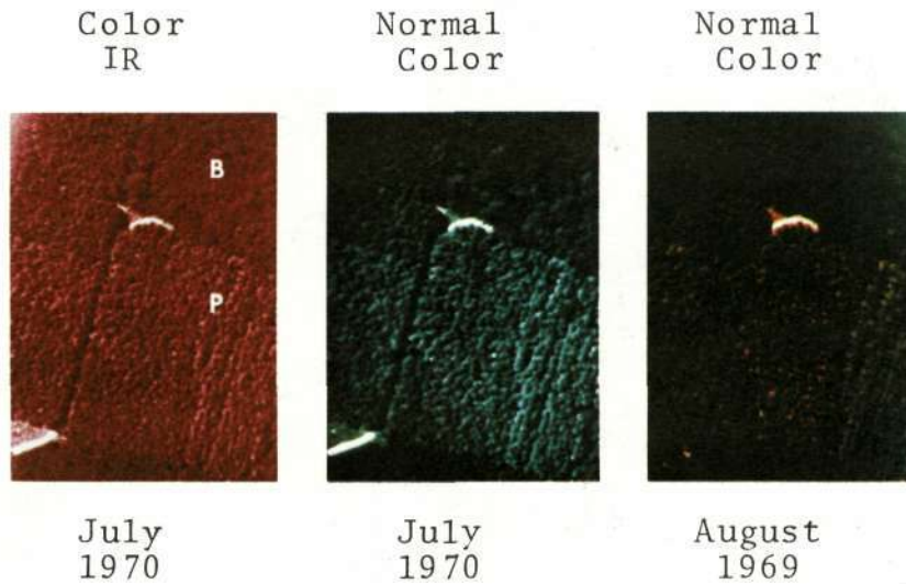
Figure 5. Needle cast on Scots Pine was much more severe in 1969 than in 1970 as indicated by these photographs taken from 3,000 feet. The brown trees in the August 1969 photo are severely infected. Note that the broadleaved (B) and pine (P) trees in the Color IR photo show nearly equally red tones.
