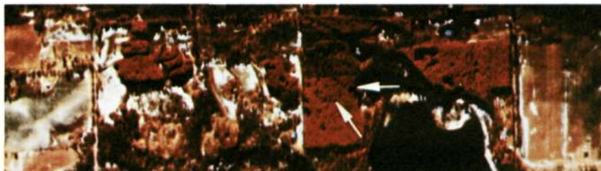
Figure 7. Simulated Color IR image prepared from data obtained with the University of Michigan multispectral scanner. The small holes in the crown canopy indicated by arrows are centers of infection by Fomes annosus .
