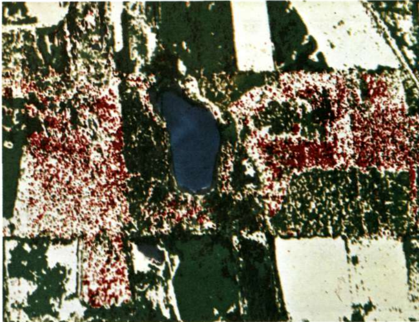
Figure 3. Recognition map of Saginaw Forest generated by the University of Michigan Spectral Analysis and Recognition Computer (SPARC). Conifers are shown in green, ring-porous species in red, and diffuse-porous species in black.
