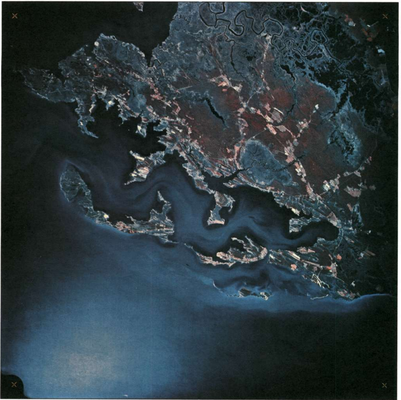
Figure 2--Coastal wetland area as photographed from 60,000 feet with a 6" focal-length mapping camera in color infrared (NASA photo).
