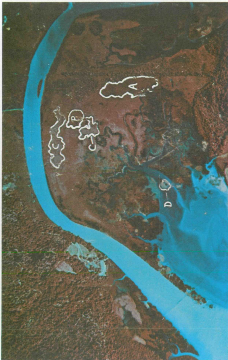
Fig. 6. Color IR photograph showing tonal quality of important wetland species. A - cattail; B - sweetflag; C - wild rice; D - water lily. Scale 1 cm = 120 meters.
