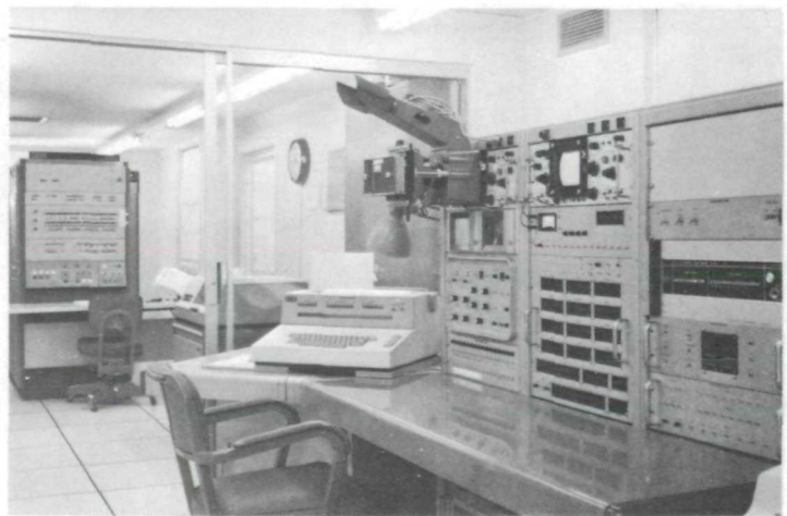
Figure 3. - Visibility Laboratory Interactive Image Manipulation Computer Facility. IBM 360/44 in left background. Interactive input-output console in right foreground.
