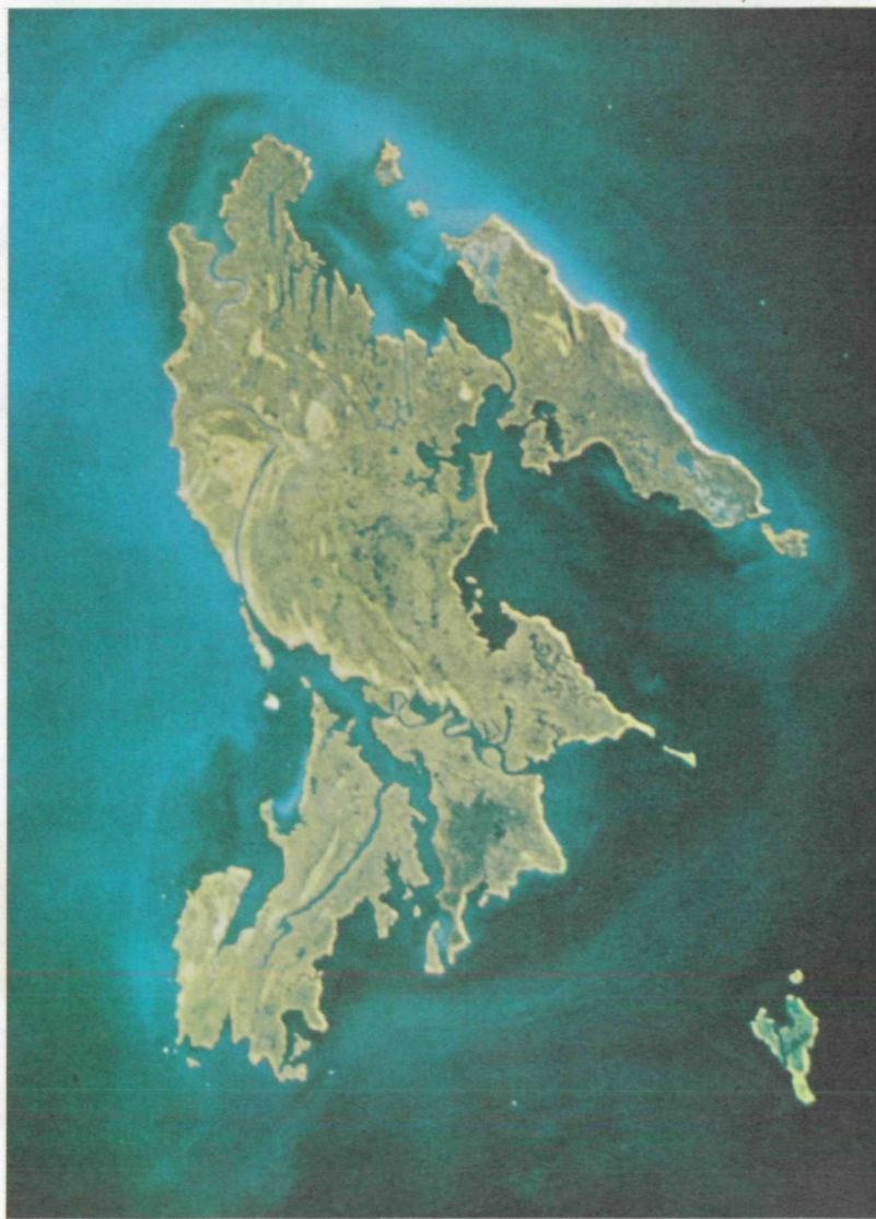
Fig. 11. High altitude photograph of a wetland showing distinctive features of high marsh (brightly colored) and low marsh (dull green color). Ektachrome color IR. Scale, 1 cm = 640 meters.
