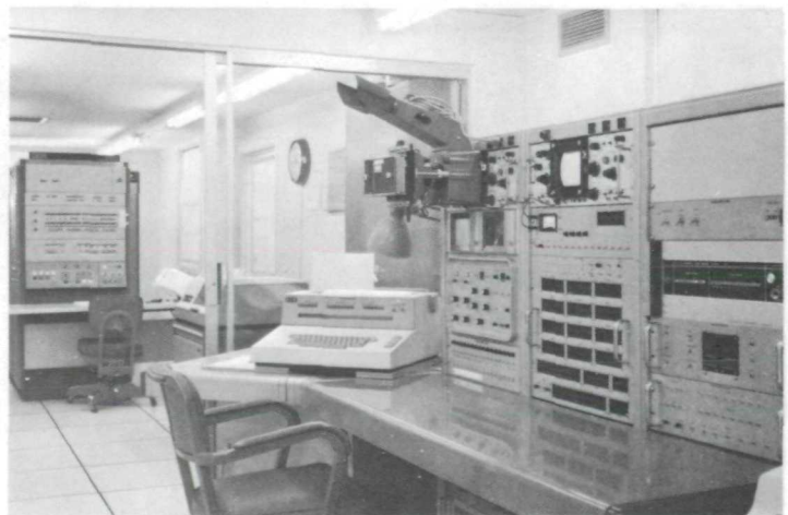
Figure 3. - Visibility Laboratory Interactive Image Manipulation Computer Facility. IBM 360/44 in left background. Interactive input-output console in right foreground.
