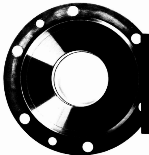
Figure 11. - Suction housing of NaK pump showing scratches.
