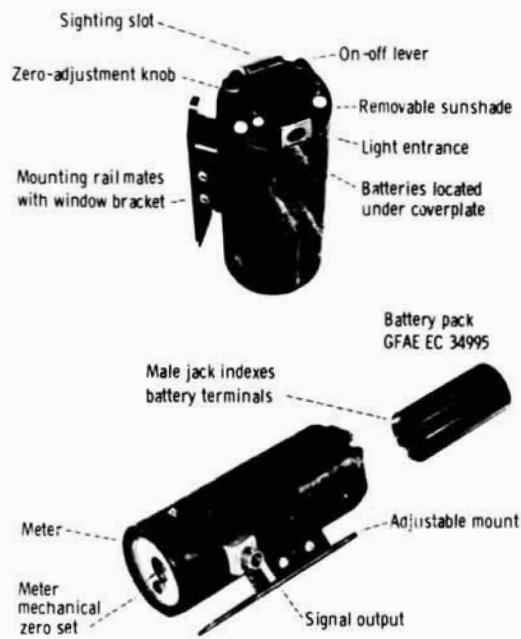
Figure 15. - Components of inflight photometer.
