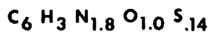
Figure 12-5.- Elemental analysis of black intumesced polymeric foam formed from p-nitroaniline bisulfate at 482° F.
