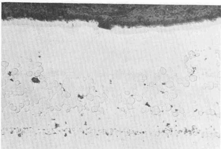
FIGURE 27. ALUMINIZED MODIFIERS NC-15, NC-16 AND NC-17 ON W-11 COATED TD-NiCr; Modifier Fired at 2375° F (Magnification: 250X)
