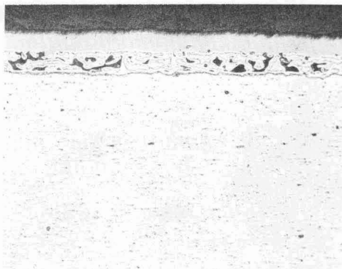
FIGURE 8. Al 2 O 3 + Ta DIFFUSION BARRIER ON TD-Ni AND TD-NiCr; Discontinuous Al 2 O 3 + Fused Salt Ta Plated
