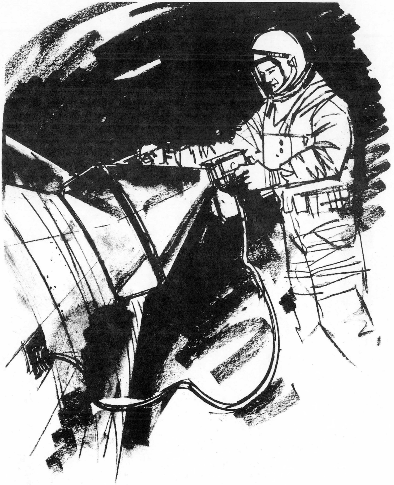
Figure 7. Space-Station Surface Re-coating Maintenance by Thin Film Deposition in Space
