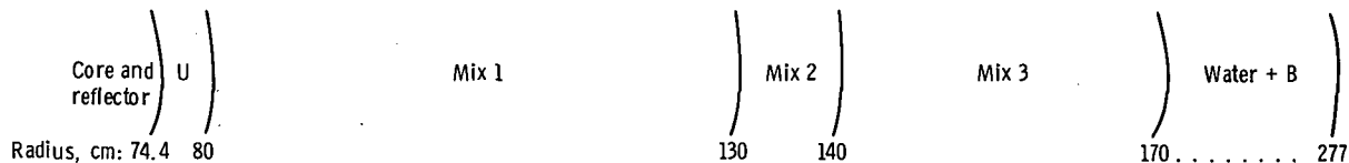
(b) Optimum shield. Reactor radius, 74.4 centimeters; shield weight, 159 000 kilograms (350 000 lb).
