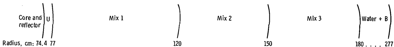
(a) Standard shield. Reactor radius, 74.4 centimeters; shield weight, 163 000 kilograms (360 000 lb).
