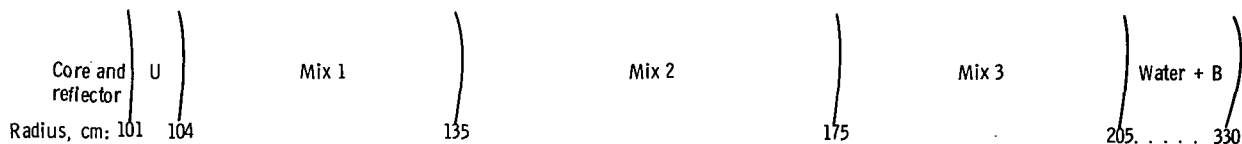
(a) Standard shield. Reactor radius, 101 centimeters; shield weight, 252 000 kilograms (557 000 lb).
