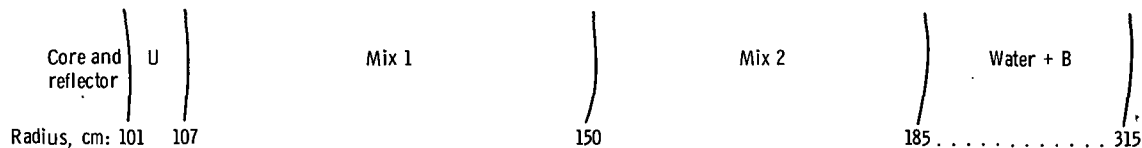
(b) Optimum shield. Reactor radius, 101 centimeters; shield weight, 237 000 kilograms (521 000 lb).
