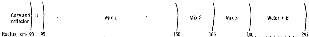
(b) Optimum shield. Reactor radius, 90 centimeters; shield weight, 202 000 kilograms (445 000 lb).
