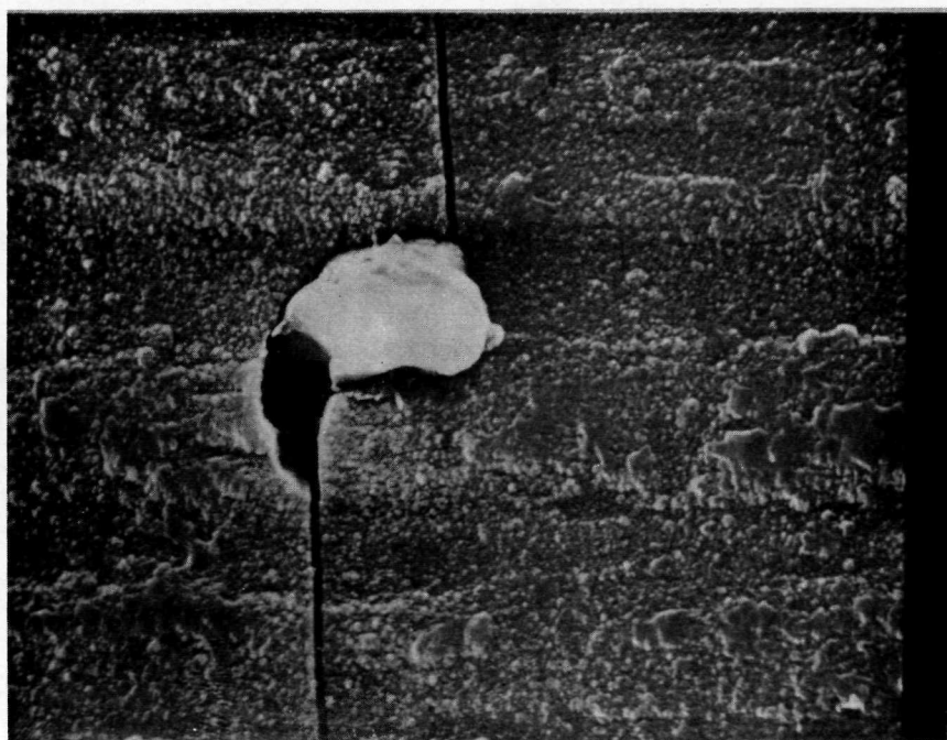
Figure 19. Defect and Crack Origin in Boron, Run 3177-12 (610 C), (x5,000)
