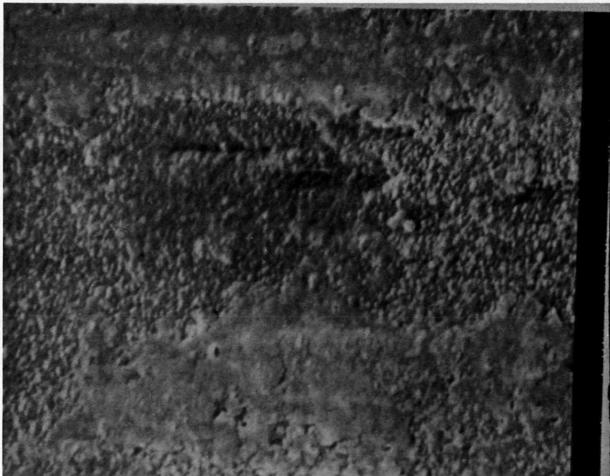
Figure 11. Boron Deposit, Run 3177-10 ( 538^{\circ}\text{C} ), with Defects (x10,000)
