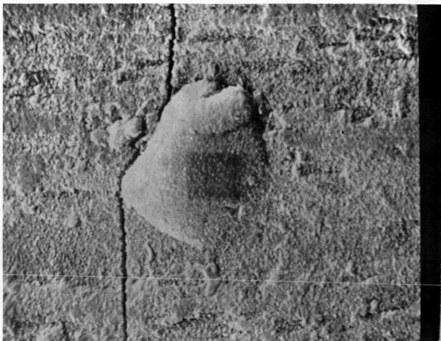
Figure 20. Crack Origin in Boron, Run 3177-10, (x5000)
