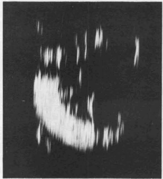
Figure 8-B Reconstructed Image Filtered by Razor Slits to Pass Elbow
