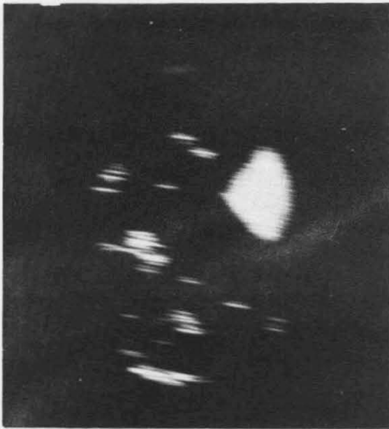
Figure 8-A Reconstructed Image Filtered by Razor Slits to Pass Pie
