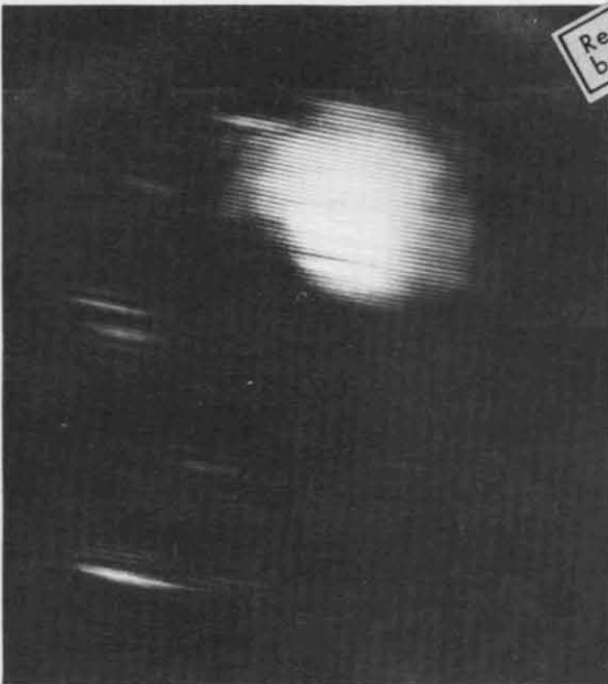
Figure 9-C Reconstructed Image Using Glass Slide Wedge Filters to Pass Pie
