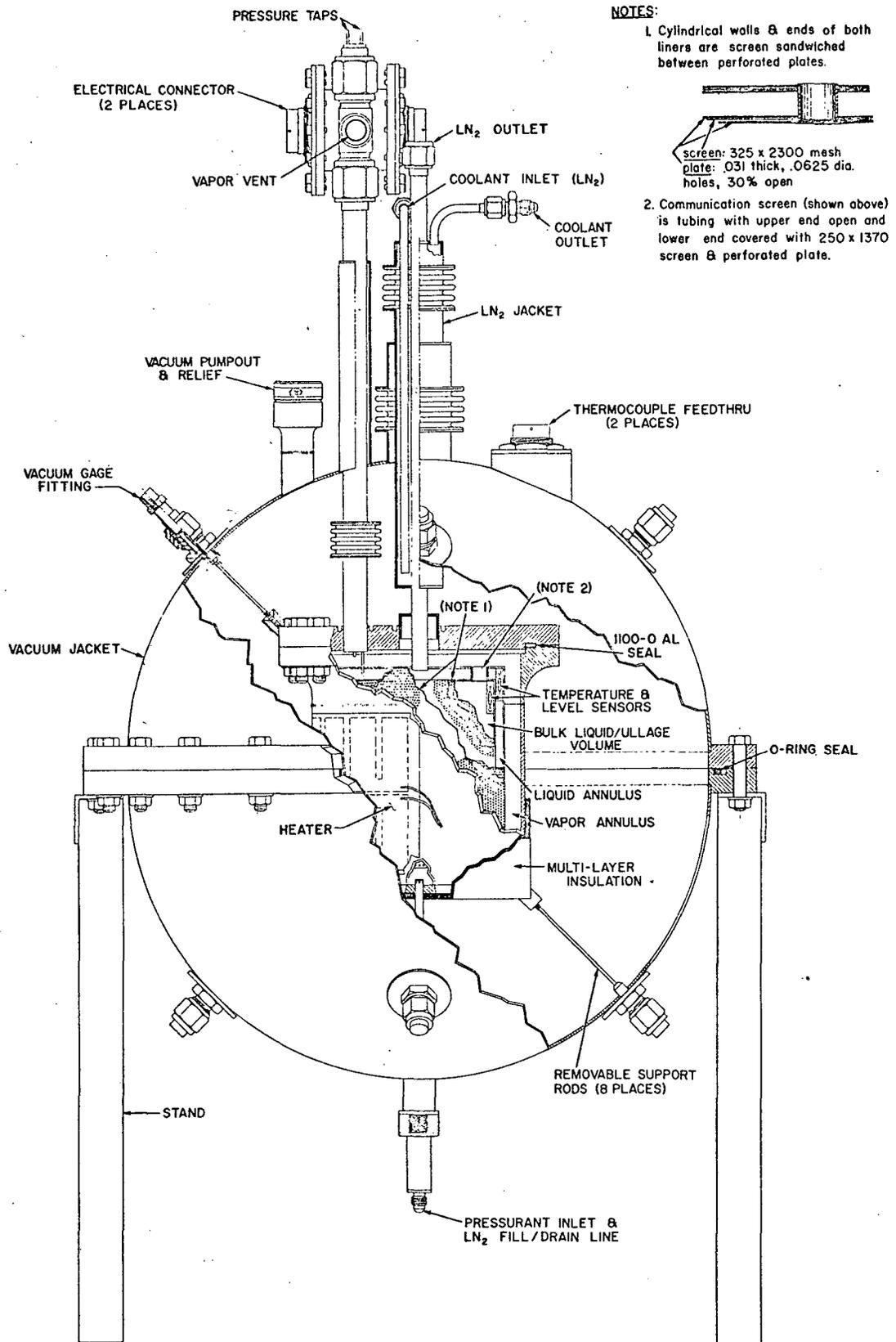
Figure 1 Cutaway View of Subscale DSL Passive Retention/Expulsion System
