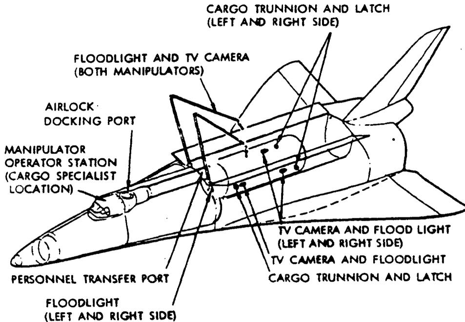
Figure 2-10. Docking and Payload Handling System
