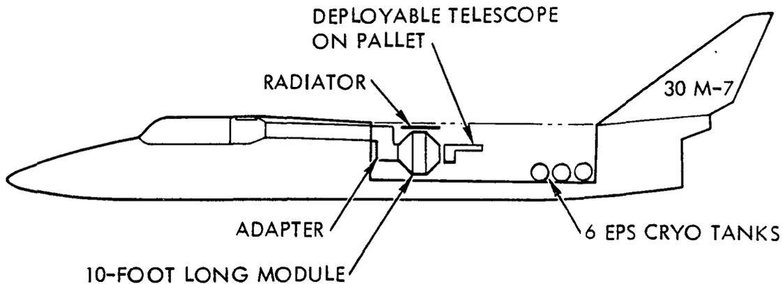
Figure 6-18. 30M-7 Payload General Arrangement
