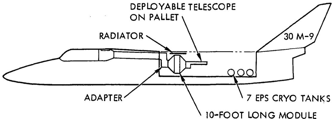
Figure 6-20. 30M-9 Payload General Arrangement
