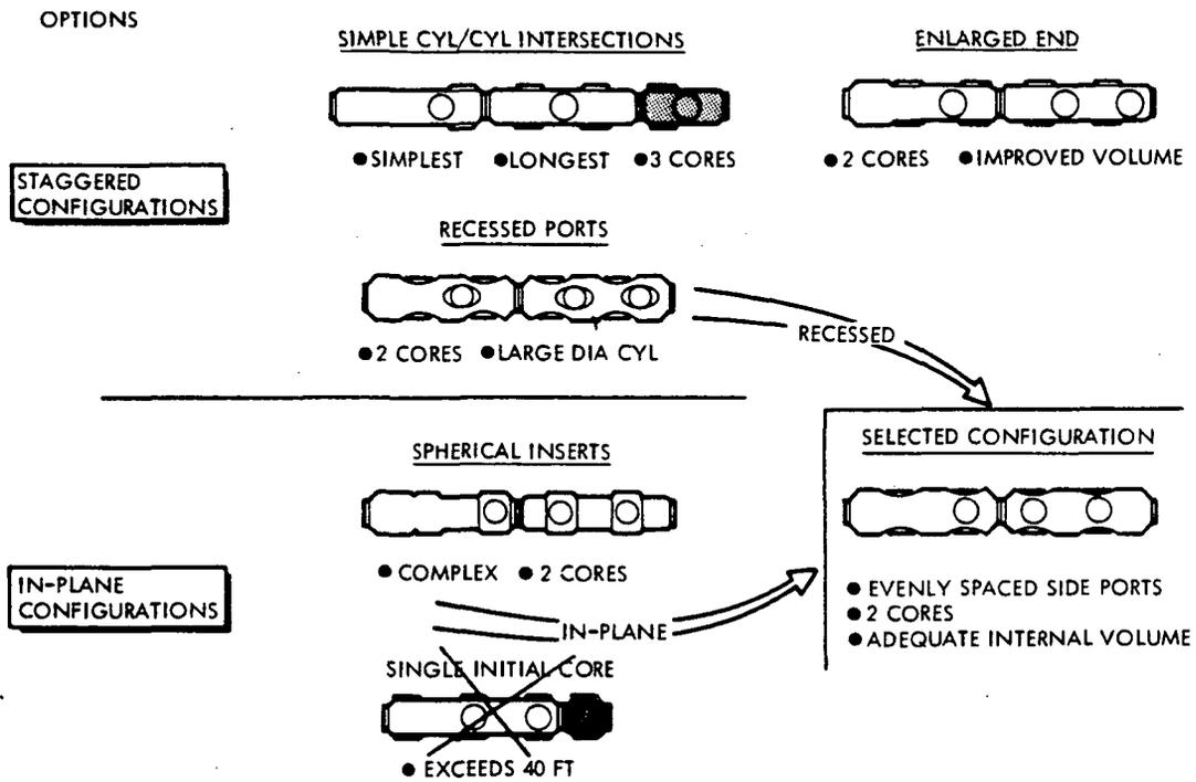
Figure 8. Special Modules (Core) Berthing Port Configuration
