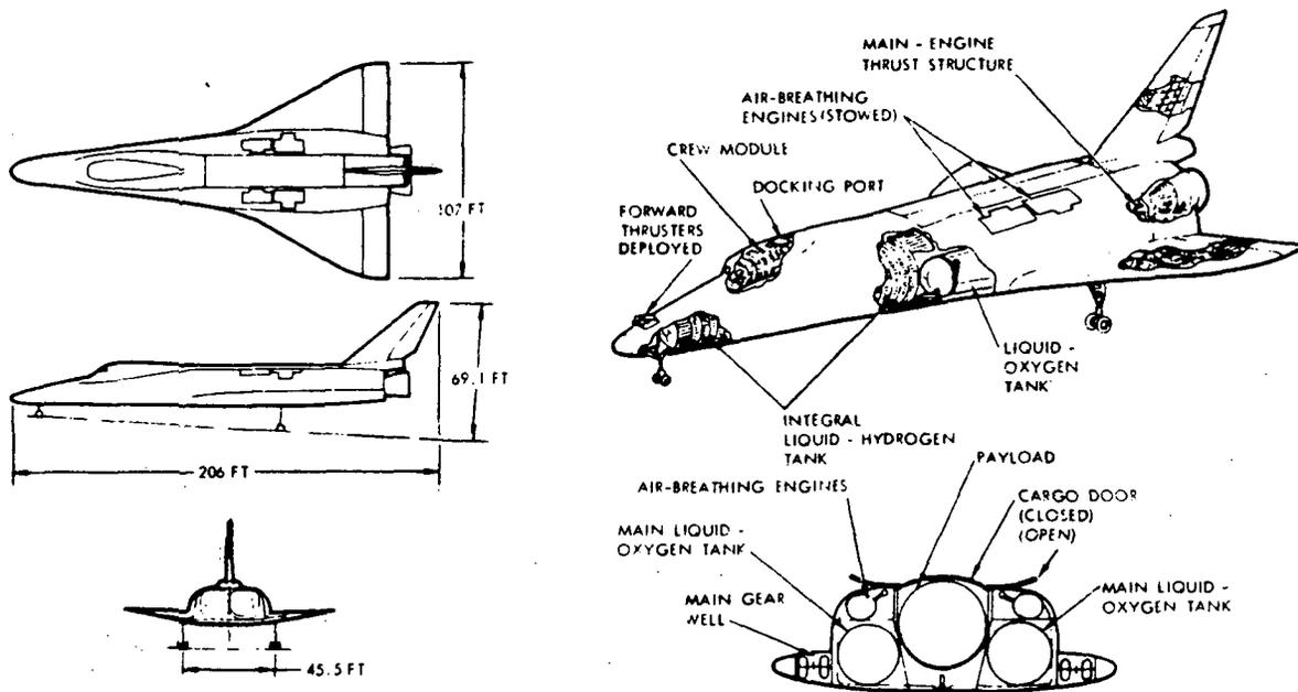
Figure 2-7. Orbiter Configuration
