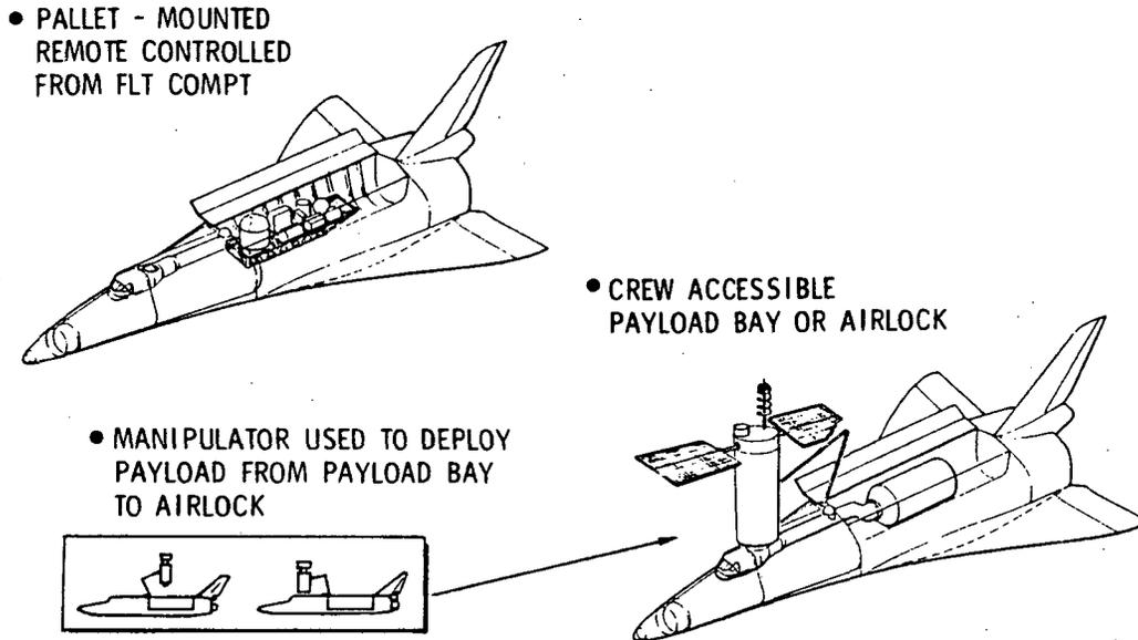
Figure 1-4. Shuttle Payload Accommodations
