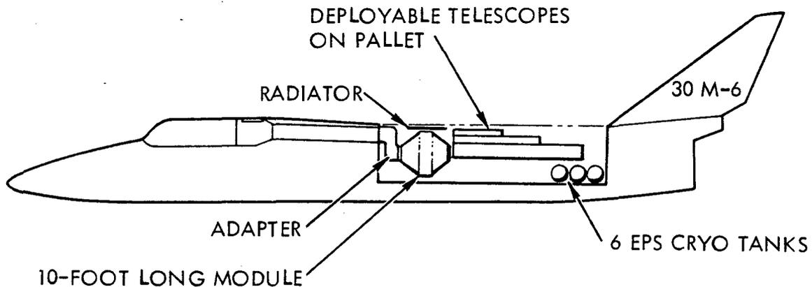
Figure 6-17. 30M-6 Payload General Arrangement
