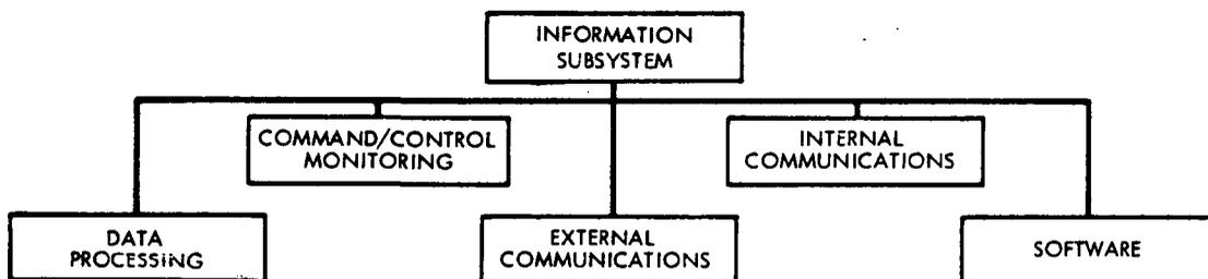
Figure 34. Information Subsystem (ISS)
