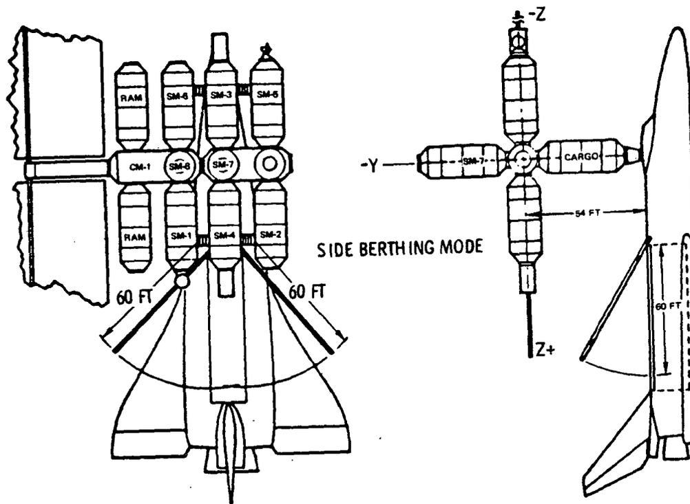
Figure 41. Shuttle/Station Berthing Mode - Initial/Growth Station, 12-Foot Diameter
