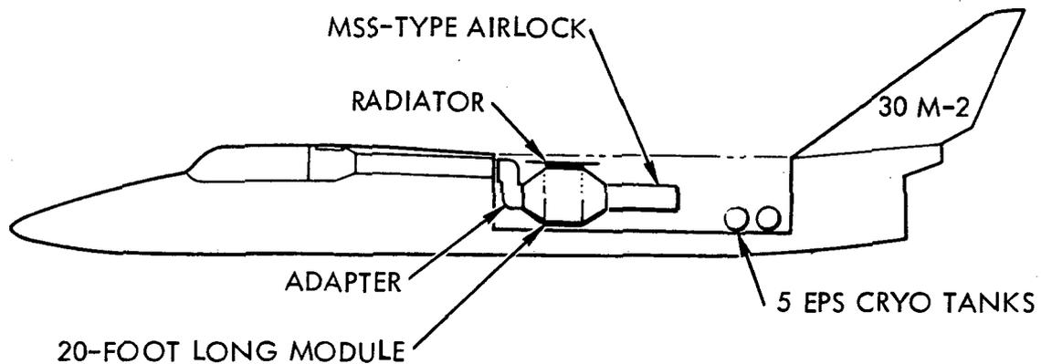
Figure 6-13. 30M-2 Payload General Arrangement
