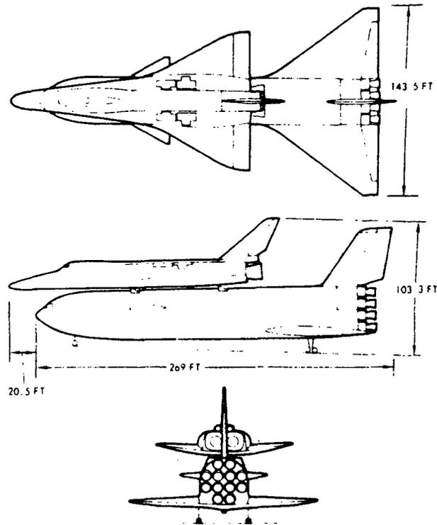
Figure 2-6. Mated Vehicle Configuration
