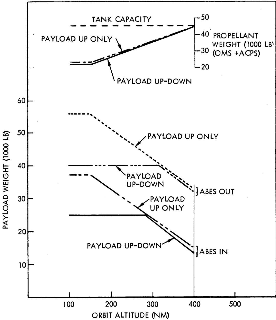
Figure 4-4. Payload Capability-Propellant Requirements:
