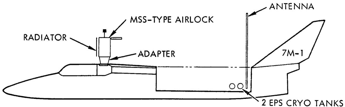
Figure 6-6. 7M-1 Payload General Arrangement
