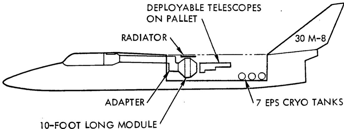
Figure 6-19. 30M-8 Payload General Arrangement
