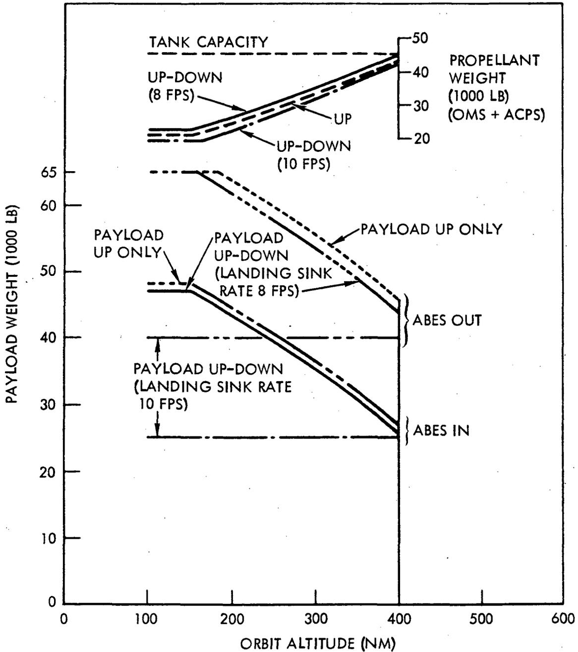
Figure 4-3. Payload Capability-Propellant Requirements:
