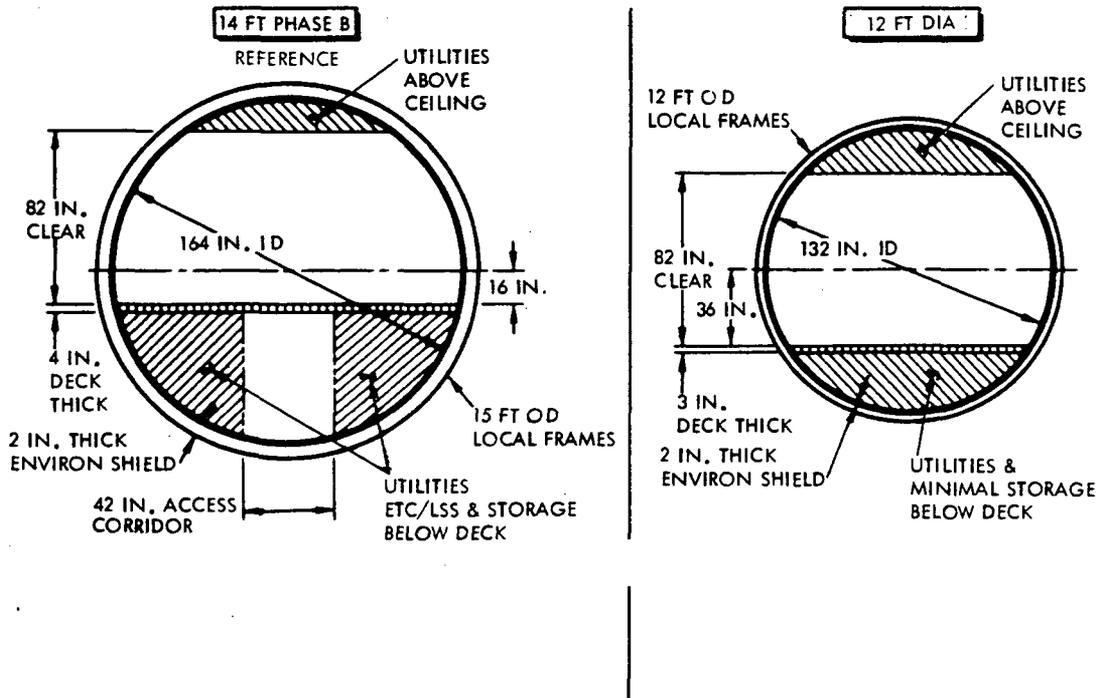
Figure 10. Station Modules - Cross Section Arrangement
