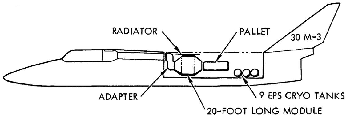
Figure 6-14. 30M-3 Payload General Arrangement
