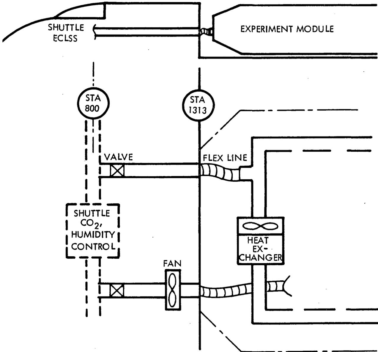
Figure 5-4. Sortie ECLSS Ducting
