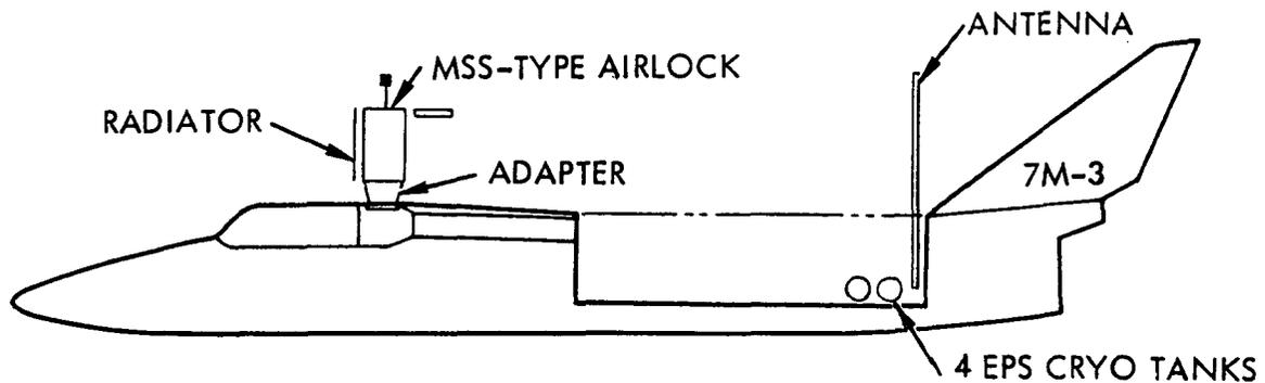
Figure 6-8. 7M-3 Payload General Arrangement
