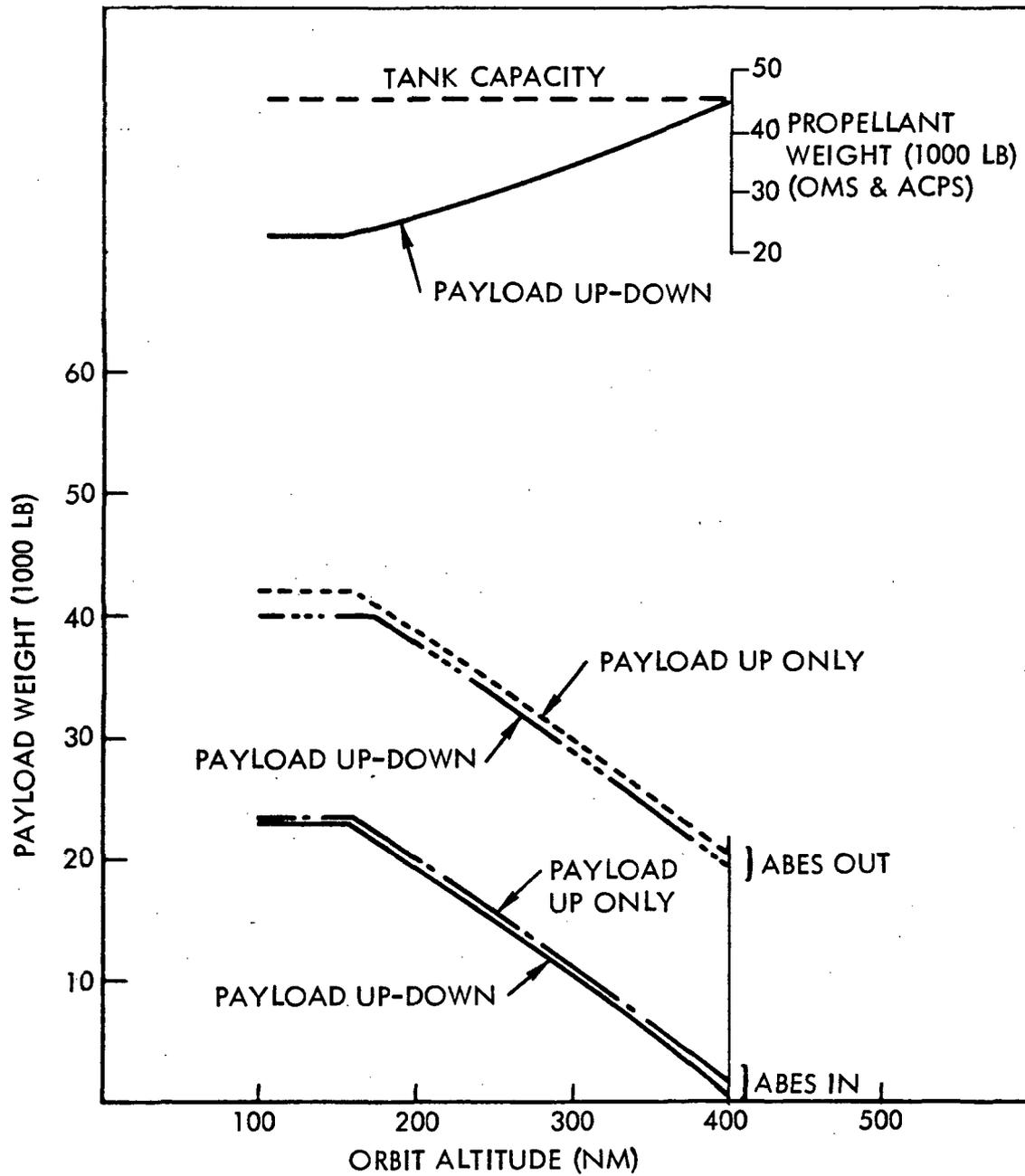
Figure 4-5. Payload Capability-Propellant Requirements:
