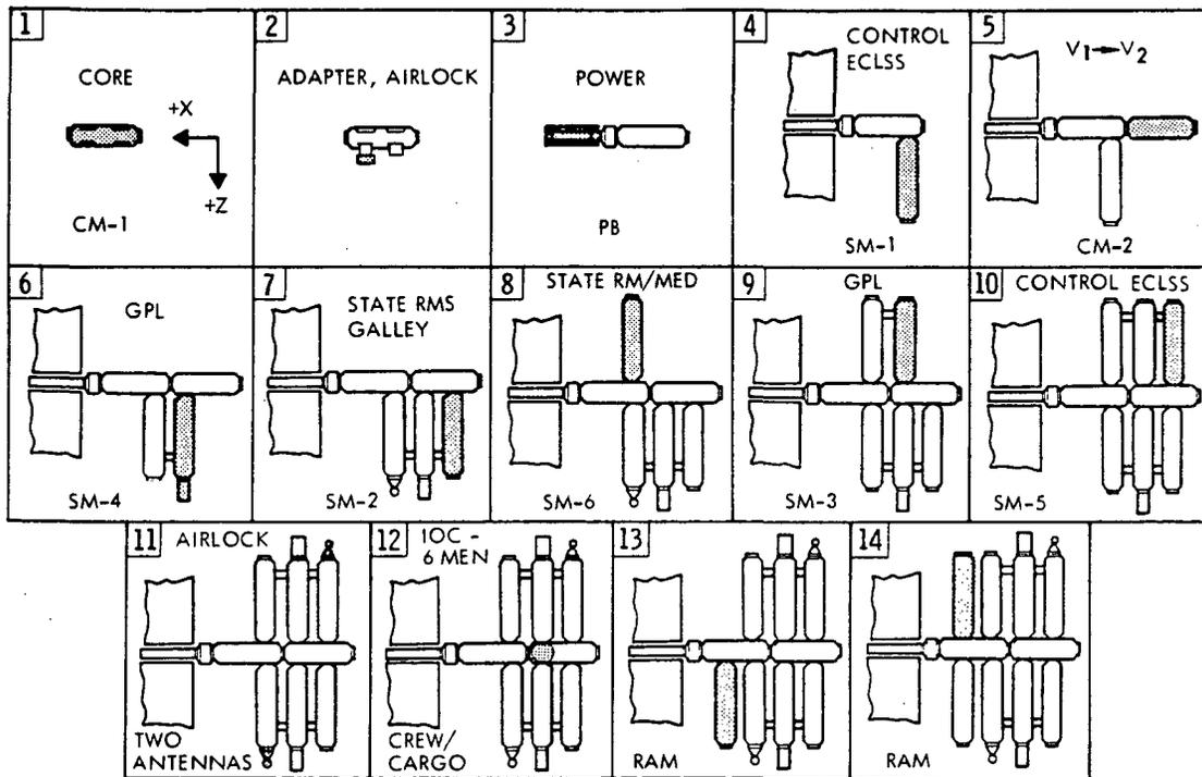
Figure 36. 12-Foot Module Initial MSS Buildup Sequence
