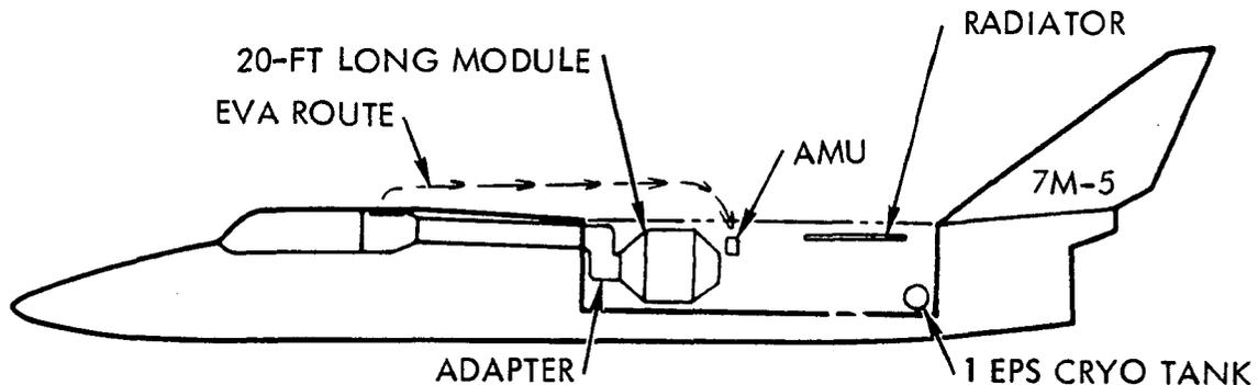
Figure 6-10. 7M-5 Payload General Arrangement
