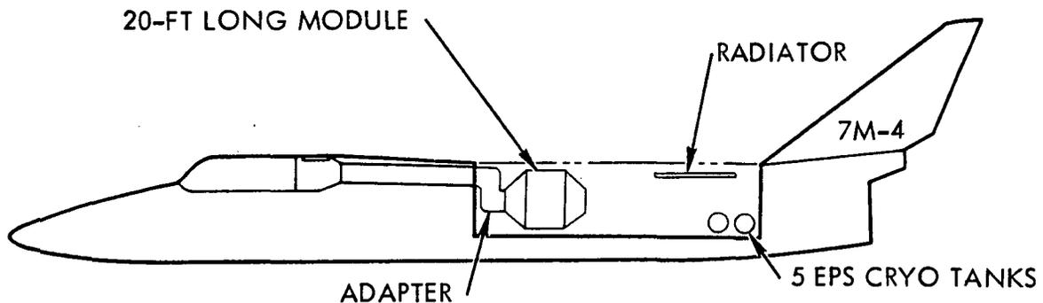
Figure 6-9. 7M-4 Payload General Arrangement
