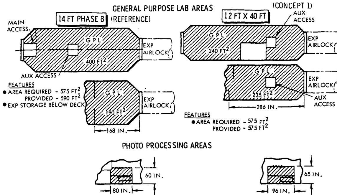
Figure 16. Station Module Facilities - General Purpose Area
