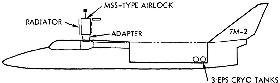
Figure 6-7. 7M-2 Payload General Arrangement
