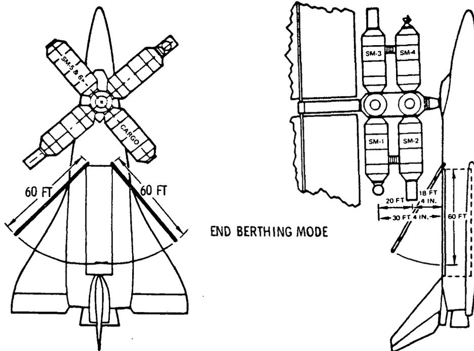
Figure 38. Shuttle/Station Berthing Mode - Initial Station, 14-Foot Diameter
