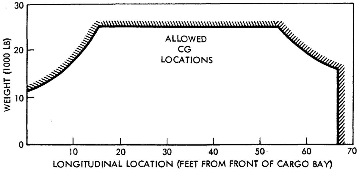
Figure 2-8. Payload Center-of-gravity Envelope
