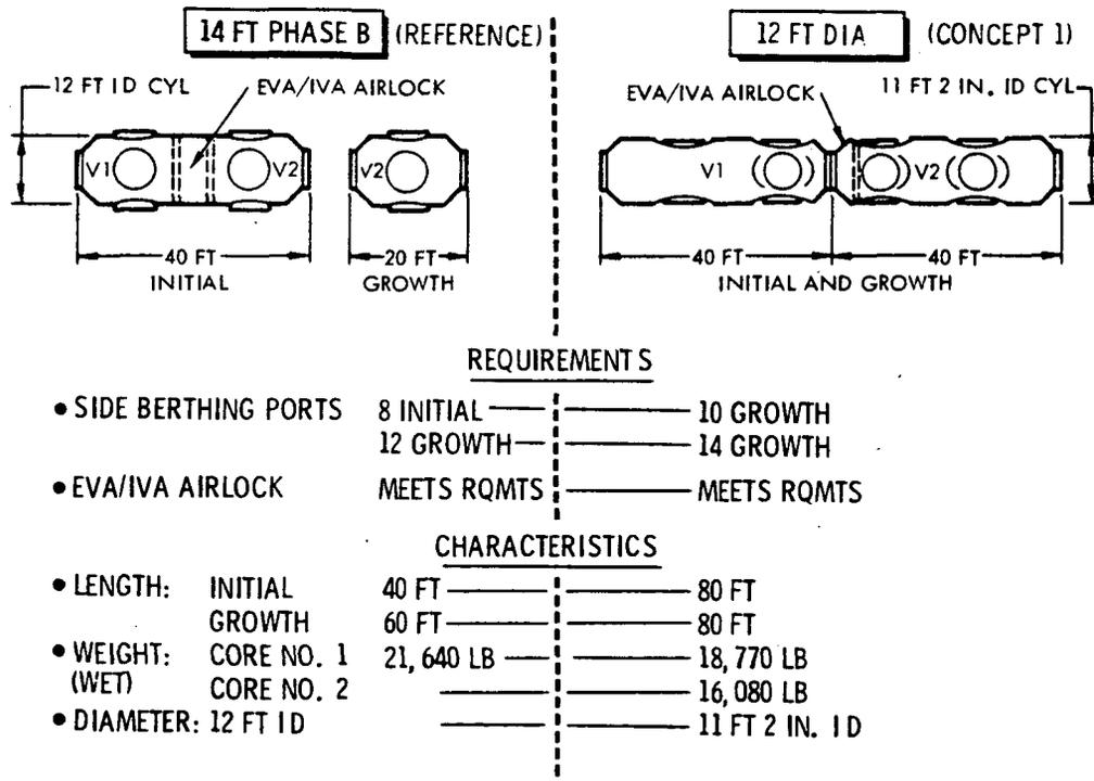
Figure 9. Special Module (Core)
