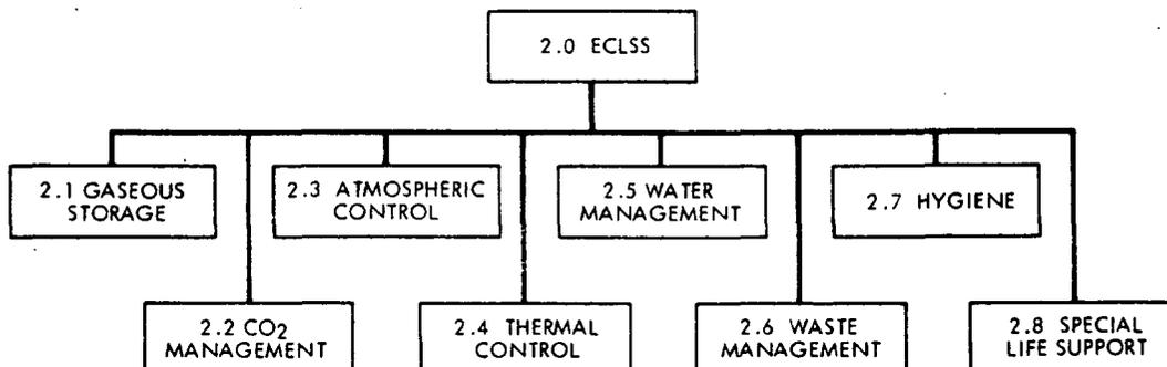
Figure 29. Environmental Control and Life Support Subsystem (ECLSS)
