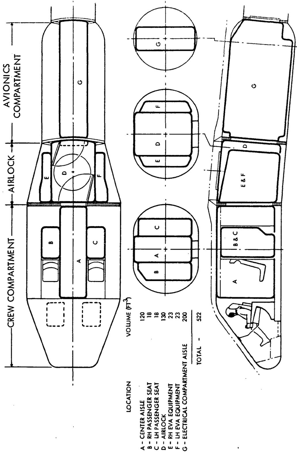
Figure 6-3. Orbiter Unused Pressure Volume
