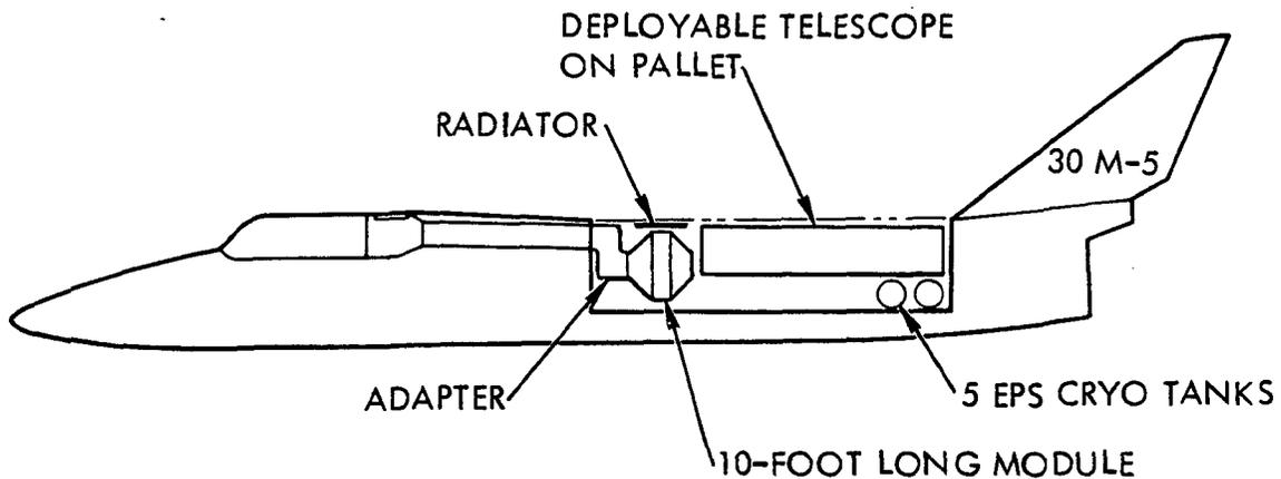
Figure 6-16. 30M-5 Payload General Arrangement
