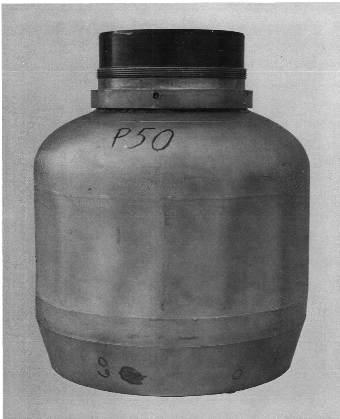
Figure 12. Buckled chamber after cooling from cure temperature
