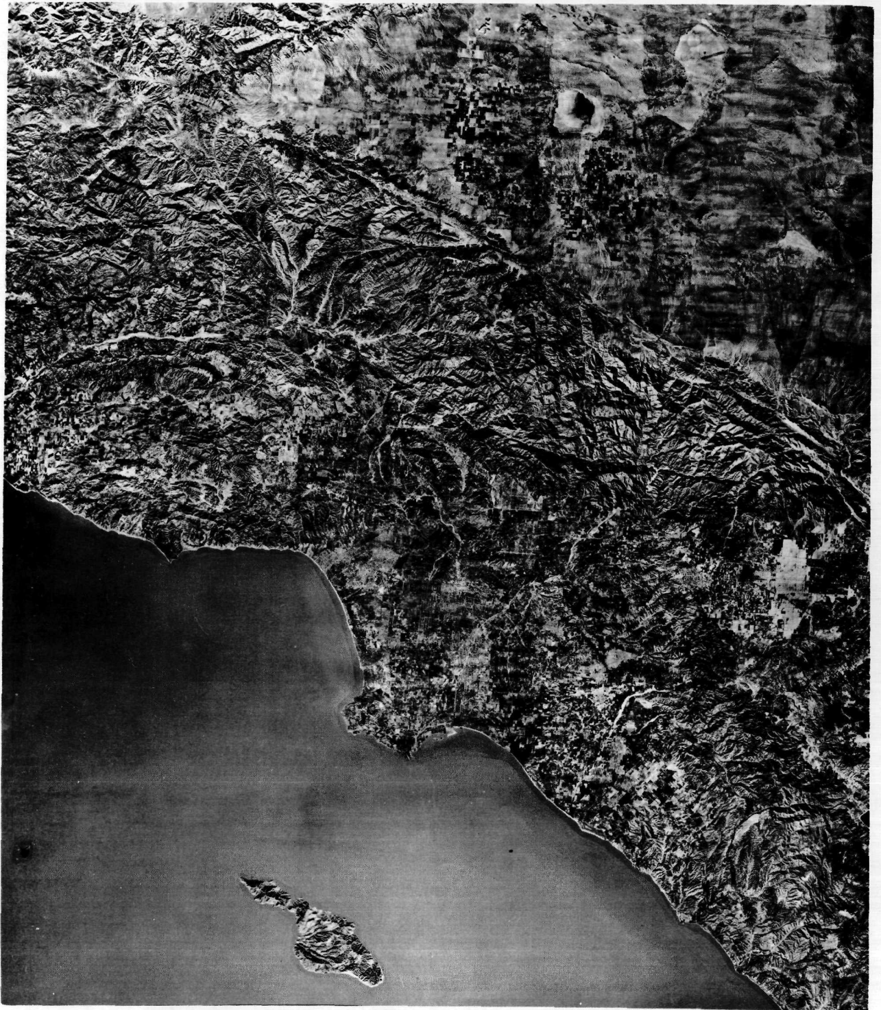
Figure 1-3 Aerial photomosaic of Los Angeles and Mojave Desert areas (Courtesy of Aero Service, Philadelphia, Pa.) (The original photomosaic constructed with hundreds of aerial photographs taken in 1953-1954 is at a scale of 1:400,000, with an estimated resolution of a few meters and covers an area of 100 x 135 miles. Santa Catalina Island is visible near the bottom. Part of the Mojave Desert is located in the upper half of the mosaic. The scar-like feature that runs diagonally from the top left corner to the right side of the image is the San Andreas fault line dividing the southern end of the Mojave Desert from the San Gabriel Mountains.)
