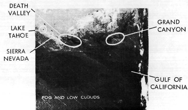
Figure 2-3 Nimbus 1 HRIR photofacsimile taken over the southwestern United States on orbit 36, near midnight on 30 August 1964. Dark shades represent warm surfaces, light shades represent cold surfaces. (Nordberg and Samuelson, 1965)
