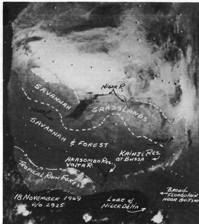
Figure 2-47 Temporal sequence of Nimbus 3 daytime HRIR showing western Africa-Niger River area. Dashed lines were subjectively drawn on these images to divide different gray level areas which roughly correspond to the savannah - forest and savannah grasslands of western Africa. The dashed-dot lines define the tropical monsoonal cloud areas.
