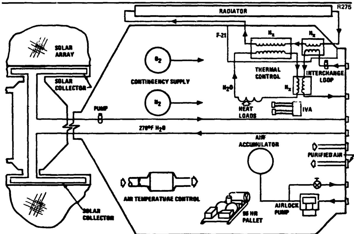
Figure 7-18. Power Module EC/LS Schematic
