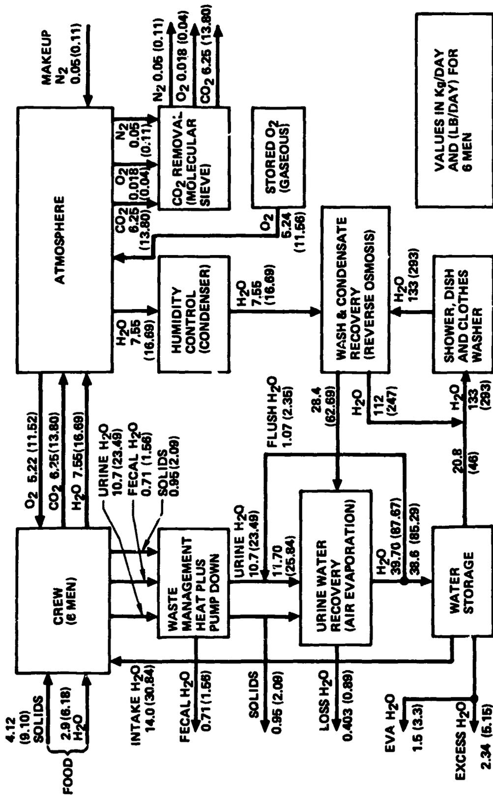
Figure 7-17. Environmental Control and Crew Support Mass Balance
