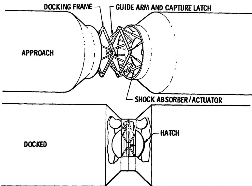
Figure 7-4. Docking Mechanism and Interface Latches
