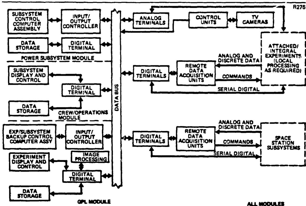
Figure 7-13. MSS Data Management Subsystem
