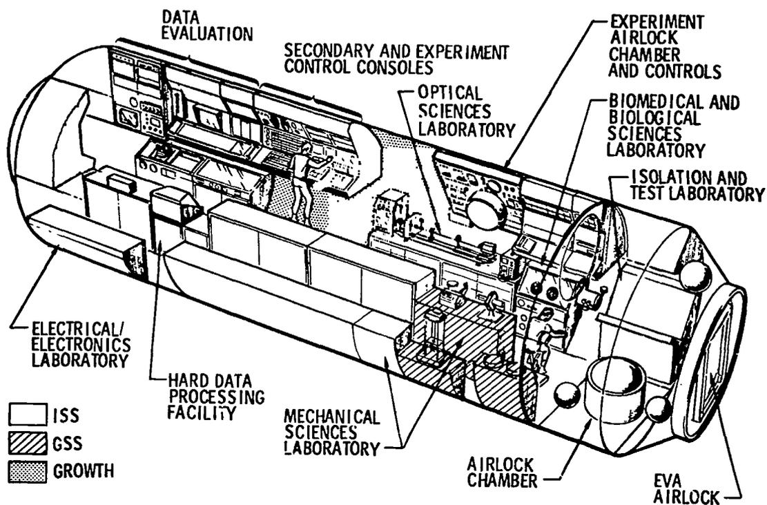
Figure 3-4. General Purpose Laboratory Module
