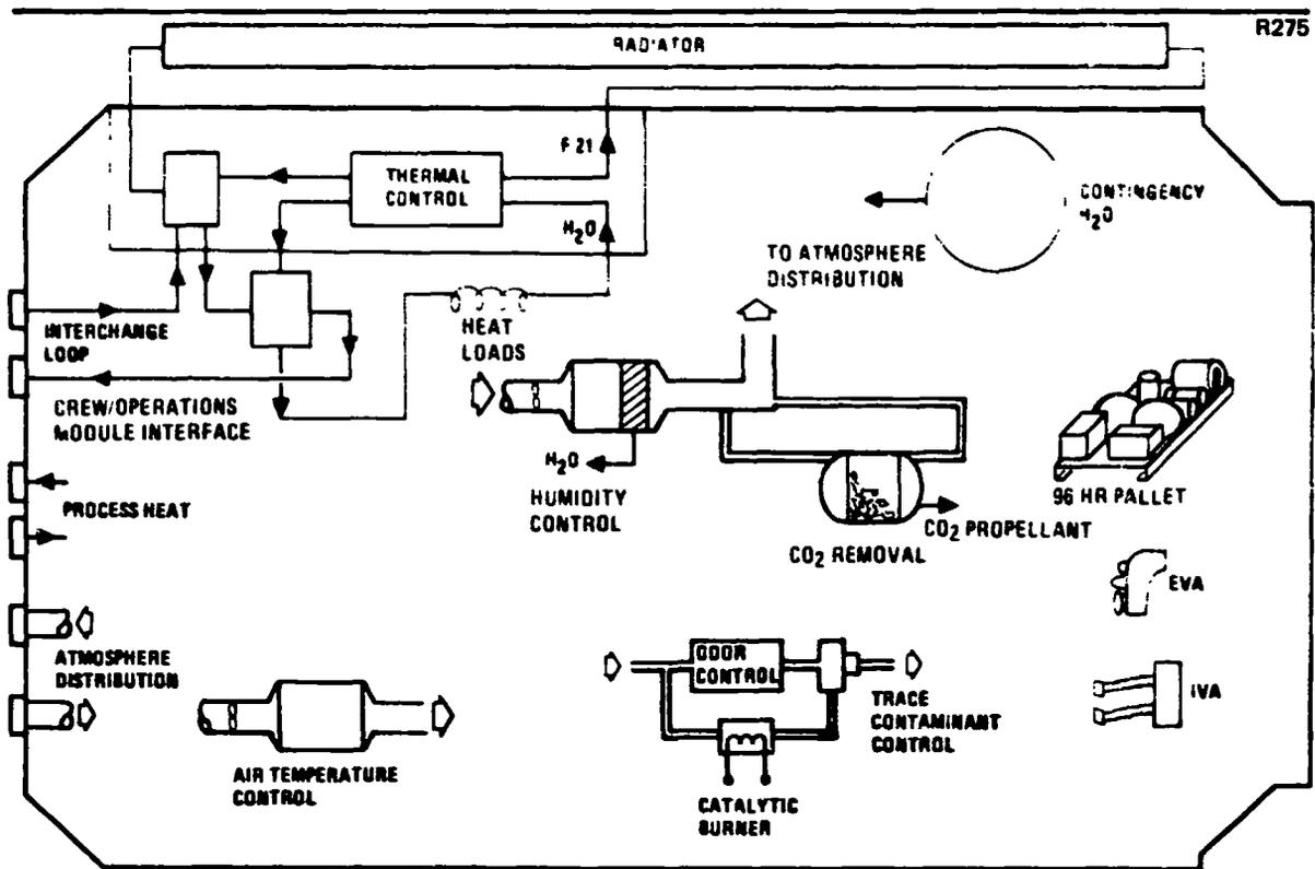
Figure 7-20. GPL Module EC/LS Schematic
