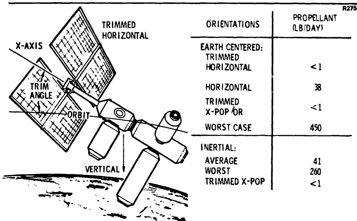
Figure 7-12. Flight Orientation
