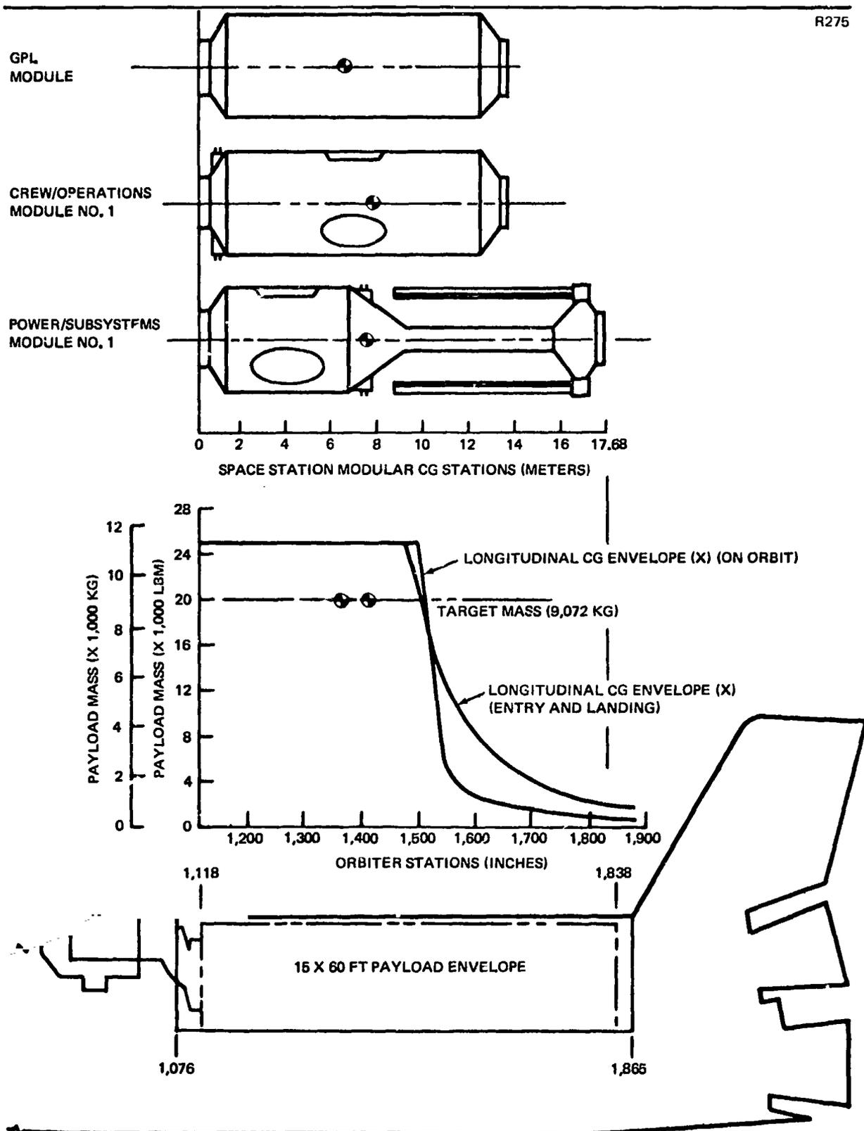
Figure 2-6. Launched Space Station Module CG's and Orbiter-Imposed Limits
