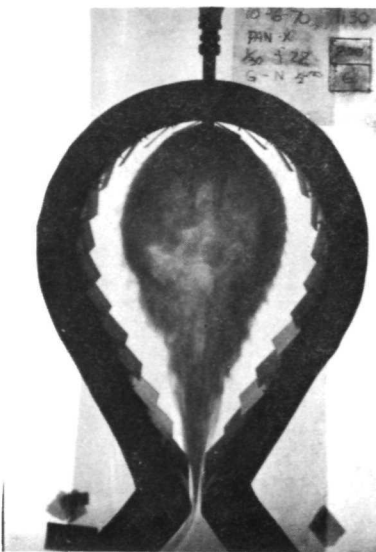
Fig. 5.11 Effect of cavity shape on flow. 200 cfm outer, 6 cfm inner
