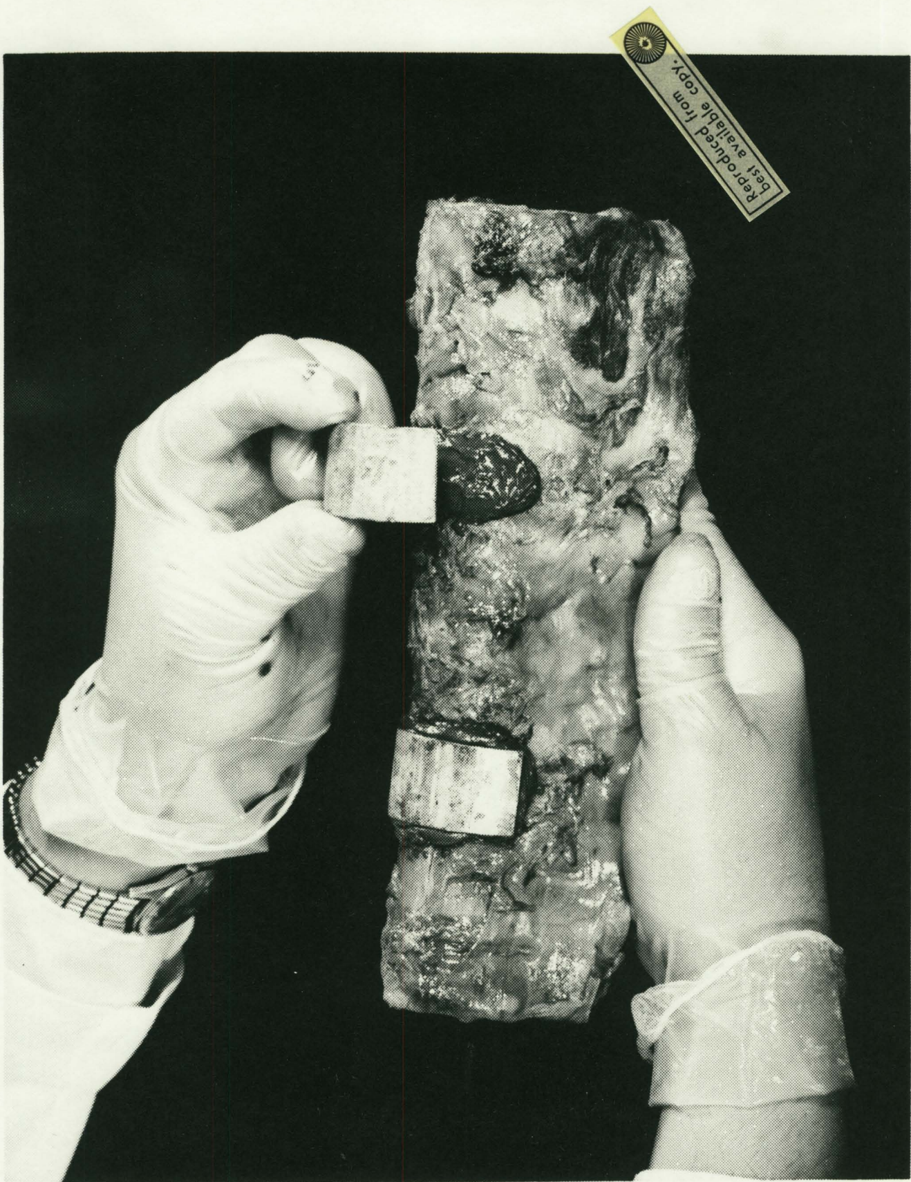
Fig. 1 Positioning of load distributing clamps on a segment of fresh, unembalmed, human vertebral column.
