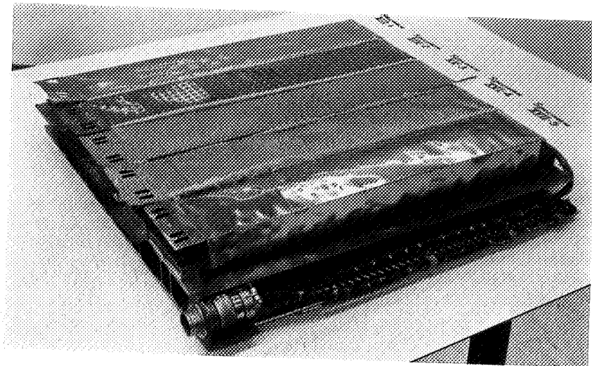
FIGURE 9 FIVE FOIL ENCASED SPECIMENS MOUNTED IN SPECIMEN HOLDER
