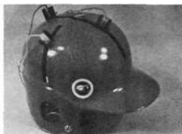
The electrodes in place in the helmet. Audiometric signals are administered via the earphones.
