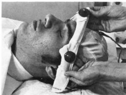
Lightweight soft cap incorporating EEG electrode developed at NASA's Manned Spacecraft Center.
