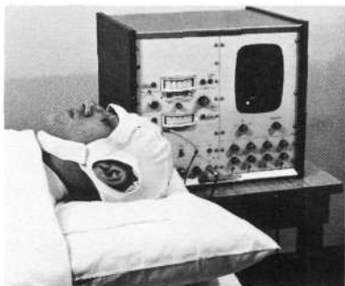
Lightweight soft cap incorporating EEG electrode developed at NASA's Manned Spacecraft Center.
