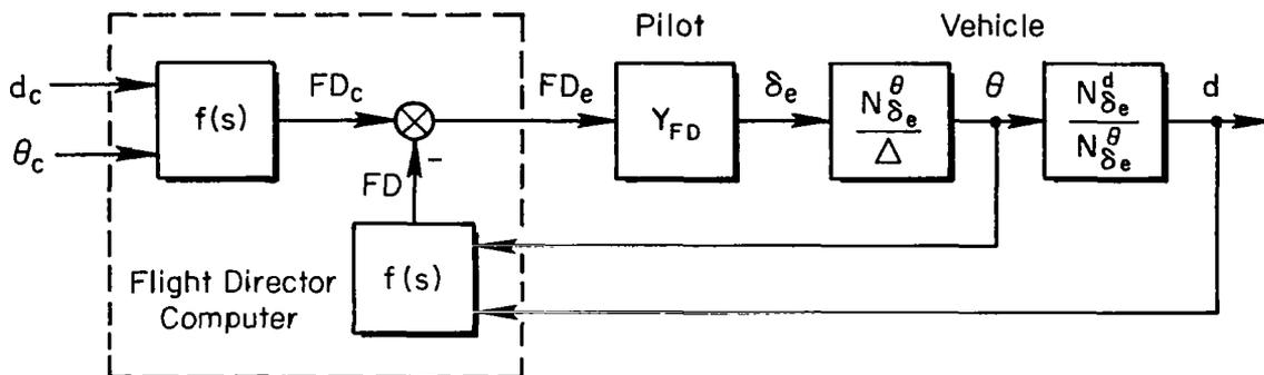
Figure 4. Flight Director Control Task, Configuration E
