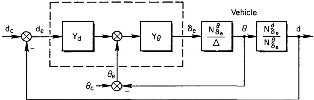
Figure 9. Multiloop System for Data Interpretation
