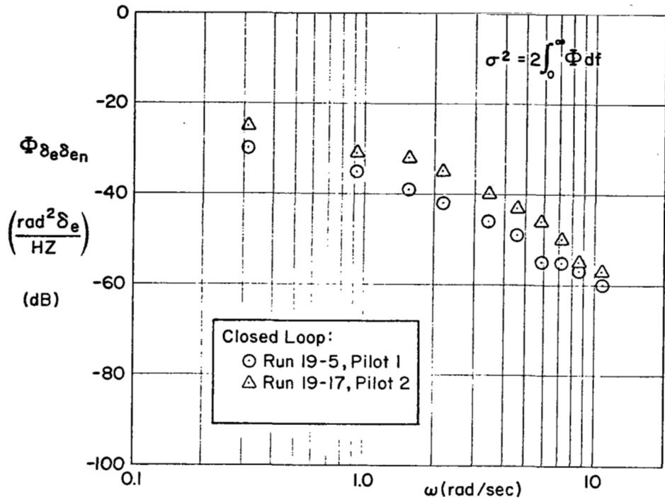
Figure 25. Remnant Spectra, Longitudinal-Only Control
