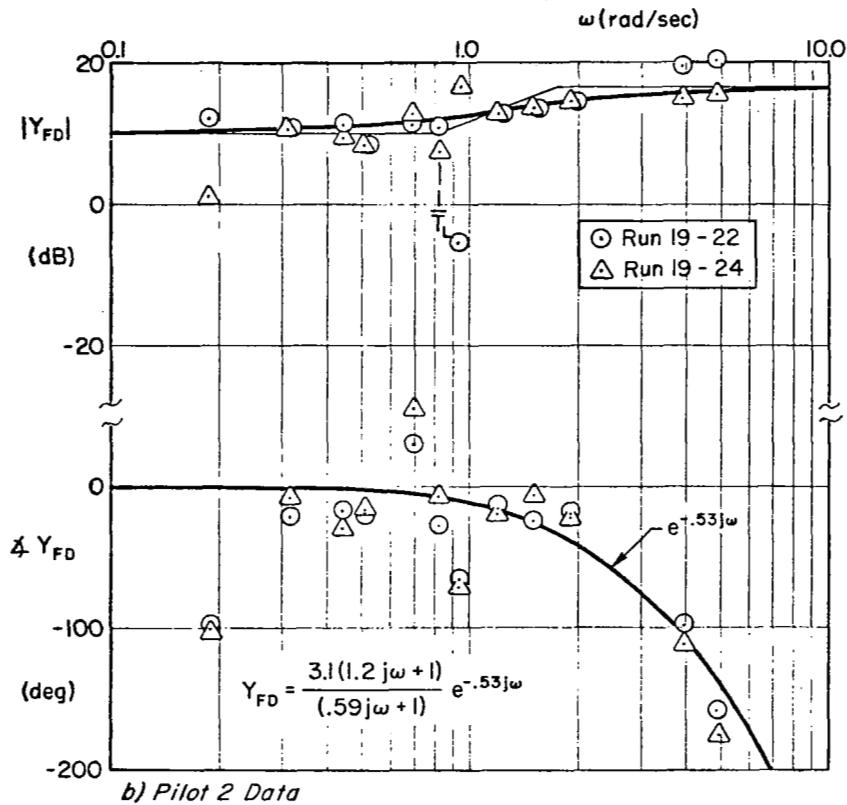
Figure 6. Pilot Describing Function for Flight Director Control
