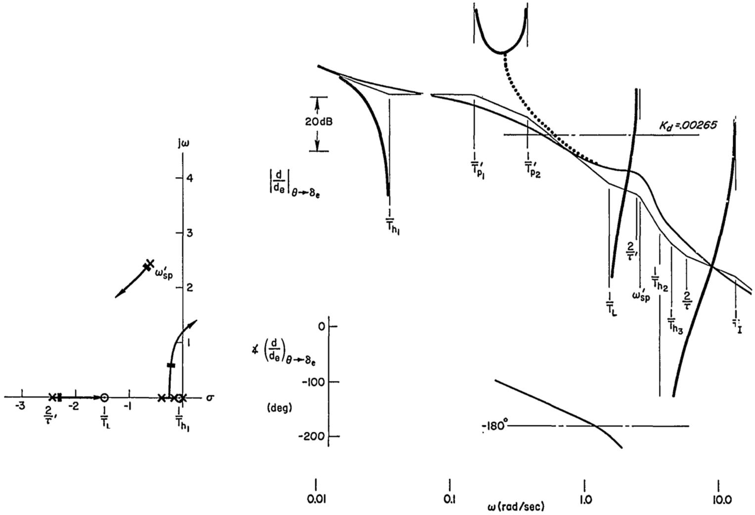
Figure B-3. Beam Deviation System Survey for Analog Pilot.
