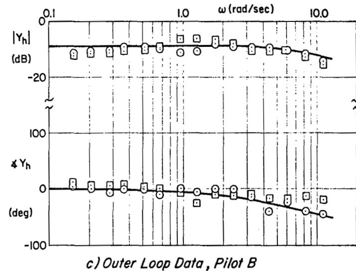
Figure 22. Pilot Describing Functions for Longitudinal Control, 1238 Study (Ref. 8)
