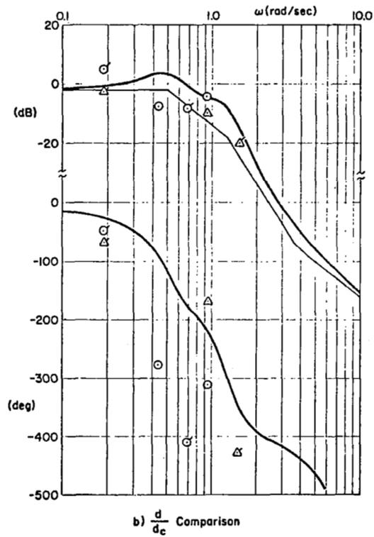
Figure 21. Closed-Loop Describing Functions for All-Axis Control, Pilot 2
