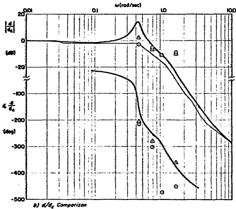
Figure 19. Closed-Loop Describing Functions for All-Axis Control, Pilot 1
