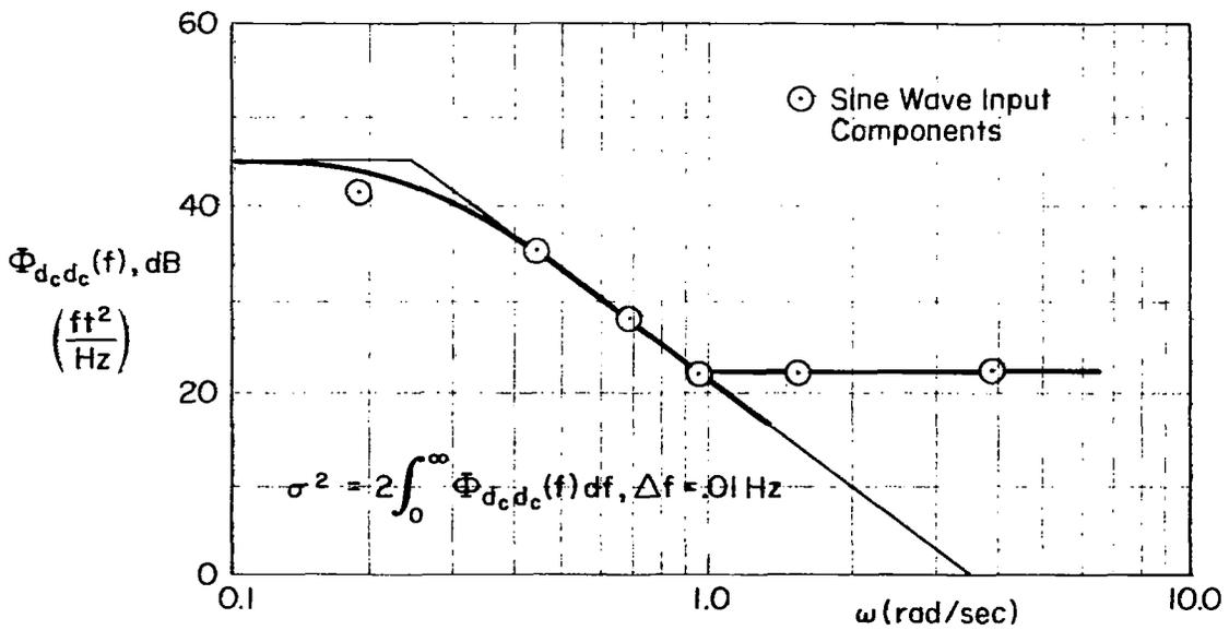
Figure A-2. Power Spectral Density of Beam Deviation Forcing Function
