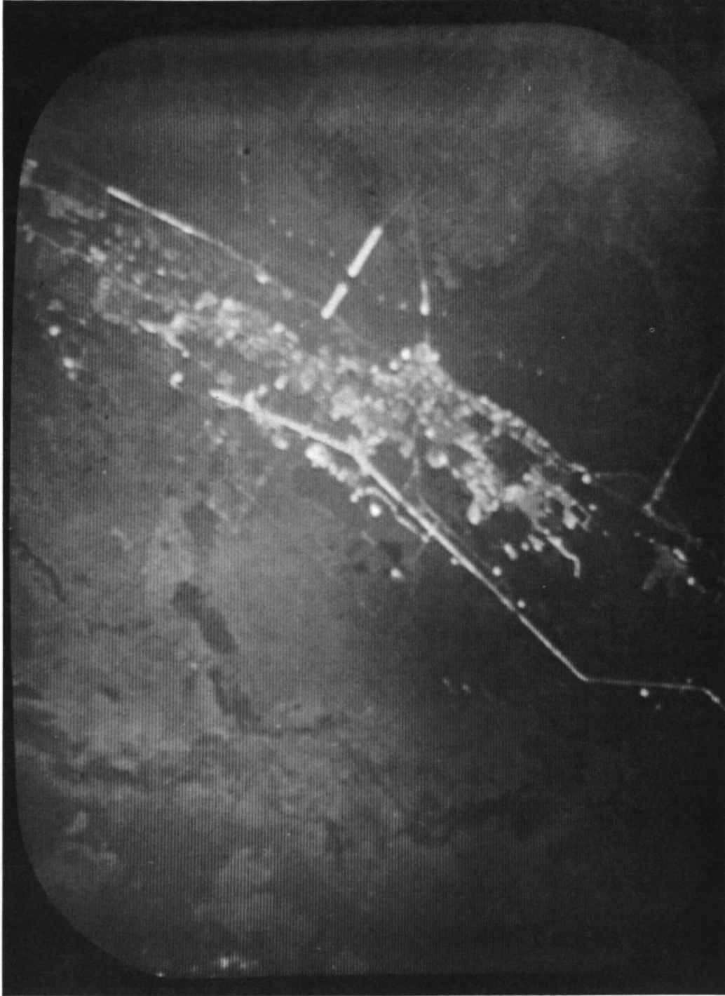
Figure 32. A 525 scan line rate simulated television image of the East Coast Florida Titusville area as displayed on a 14 inch monitor at a scale of 1:125,000.
