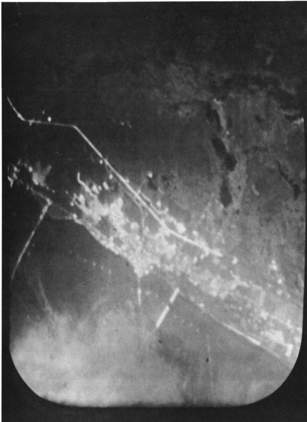
Figure 37. A 945 scan line rate simulated television image of the Titusville area of East Coast Florida as displayed on a 14 inch monitor at a scale of 1:125,000.
