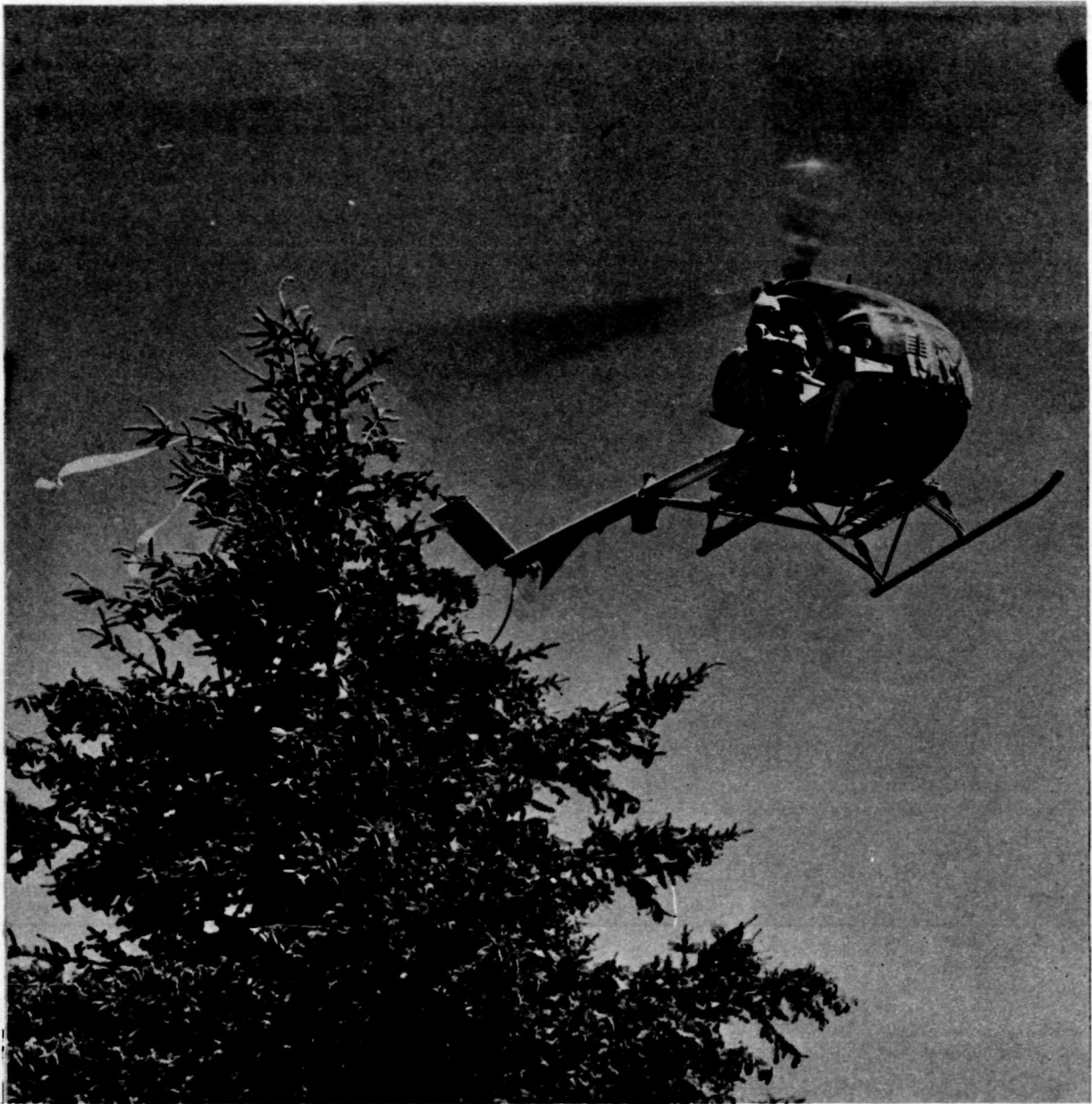
Figure 3.--Infrared heat emissions from individual trees are recorded with Barnes PRT-5 radiometer and a Cole-Parmer recorder. Helicopter is orbiting above the trees in a flat circular pattern about 150 feet above the tree-tops.
